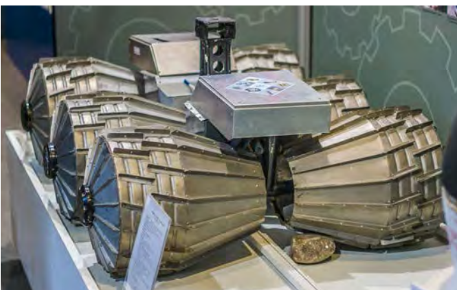
Russian Mars Rover has two independent suspensions on its front, and back. Right, the real size of space capsule.
