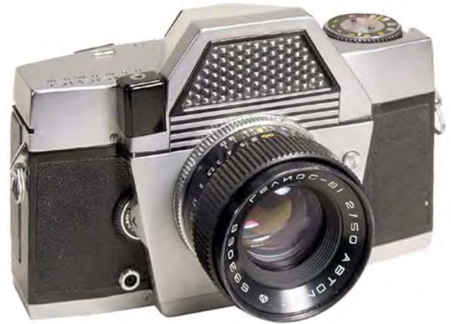
Kiev 10 35 mm Russian camera with extraordinary complex design utilizing two retractable rotary blade shutters. Standard pentaprism is utilized for reflex viewing.
