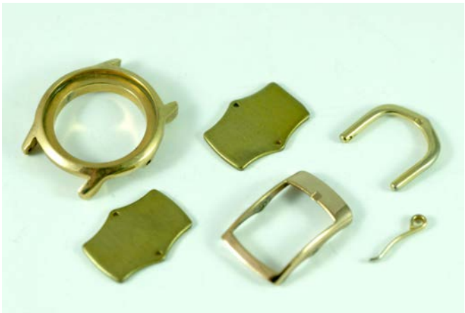
Stamping machines fabricate different parts of the watch (right). Left, the drive belt rotates a large pulley to transfer the stamping force. There is a specific stamping machine to make the rear cap of the watch from stamped out metal discs.
