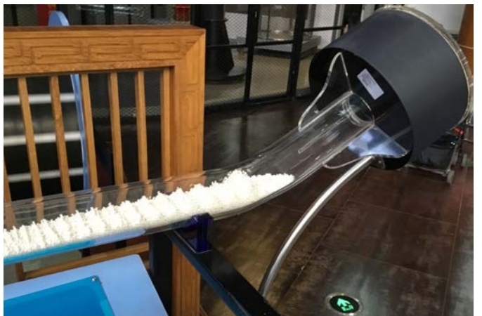
Powerful magnet at center attracts compass needles along its similar poles. China currently has a monopoly in super magnets. The audio speaker (right) produces longitudinal sound waves, visible via the floating pellets inside glass tube.
