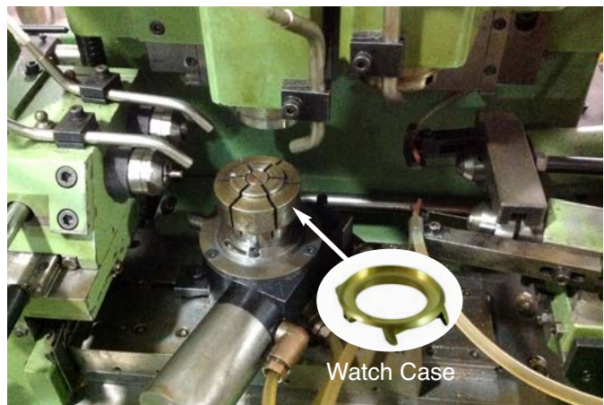
Pneumatic drilling machine (above) fabricates all the side holes on a watch case before it goes to polishing. An experienced opereator can perform all operations without looking at the control panel push buttons (for more details see Page 21)
