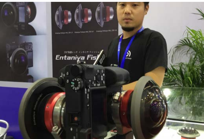
High quality fisheye lenses for the cinematography market (left) on display, with an image circle that can fill the full frame sensor format. A surface profiler interferometer (right) suitable for quick lens testing was reasonably well made.
