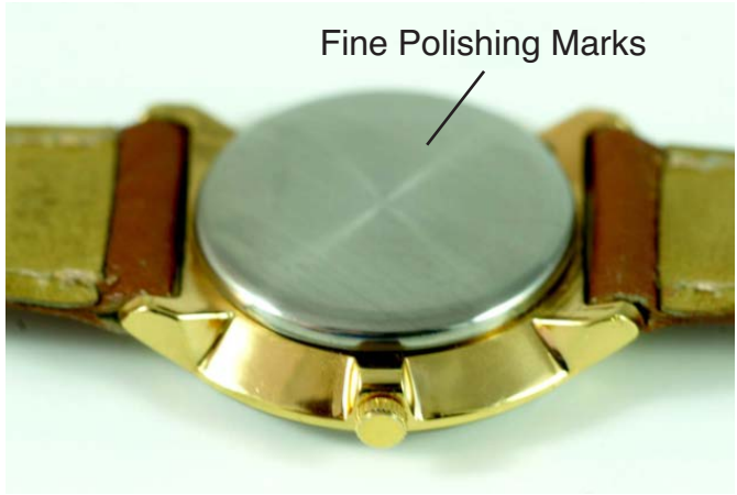
The blank rear cap is deburred, and polished with abrasive paper while it's spinning. The watch dial (right) is the most visible part of a watch. The first operation is to solder two legs on back of the dial for mounting onto the watch movement.
