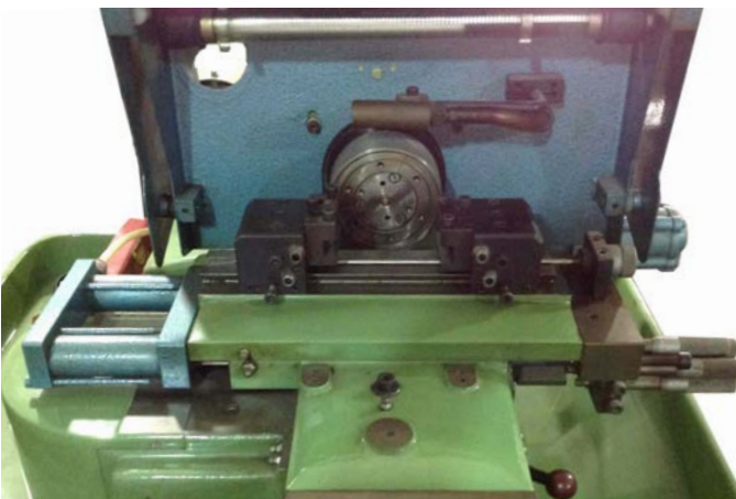
These Swiss designed machines are setup to do specific tasks on the watch case, and the operations performed are to, i.e., thread the back of the case (left) for installing the rear cap, or do other machining operations on the case (right).
