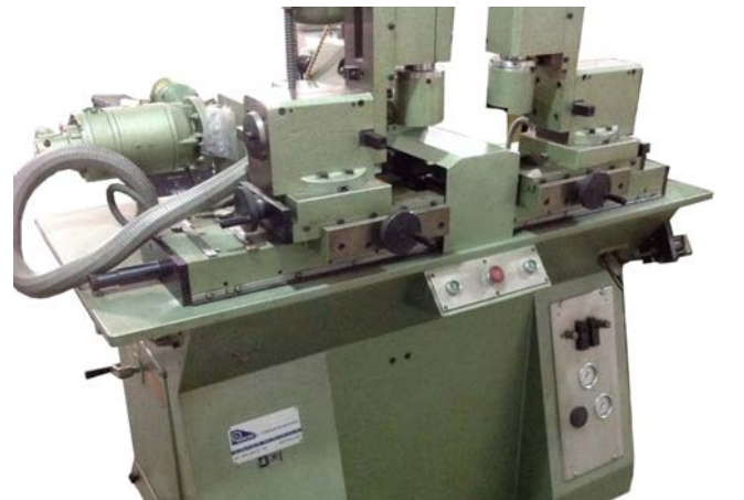
These Swiss designed machines are setup to do specific tasks on the watch case, and the operations performed are to, i.e., thread the back of the case (left) for installing the rear cap, or do other machining operations on the case (right).
