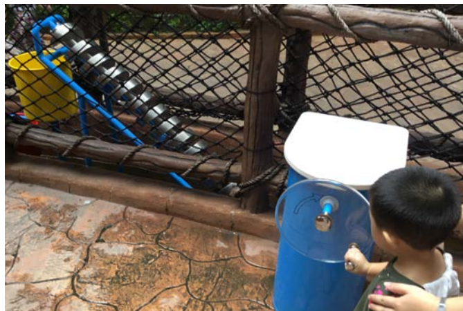
A child learns how to put a simple puzzle together (left). A hand operated water screw pump in the shape of a drill, rolls water upward (right). I have seen these made of wood before, but this one uses steel drum, and it's much easier to learn.
