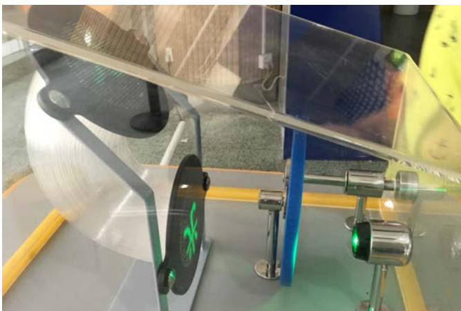
The light guide experiment utilizes a coherent fiber bundle to transfer the image. There is an image wheel that rotates by a knob on the right to change several projection targets that go through the fiber bundle to form an image.
