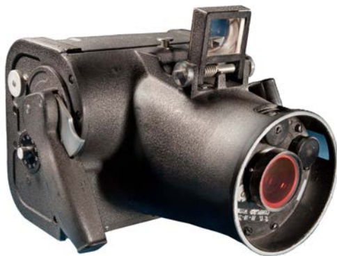
8. K-20 Aerial camera designed by Sherman Fairchild. He had numerous patents in this field to ensure film flatness across the film plane during exposure by an air suction mechanism from behind the film pressure plate.
