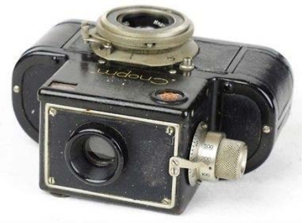
2. Sport: The first 35 mm SLR made in Russia in 1934, a year before Kine Exakta (designer unknown). It featured a reflex mirror that swung up, and a focal plane shutter that utilized single blades for the first, and second curtains.
