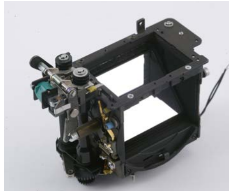
Zeiss lenses for Contax were designed by designer Dr. Erhard Glatzel (R). He designed Contax RTS lenses, while Dr. Katsuiiko Sugaya (no photos found) designed the unique Contax RTS shtter (left) with balanced curtain acceleration.
