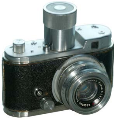
Robot spring driven camera was the go-pro equivalent camera in 1930's. It fired, and advanced the film at 2fps.
