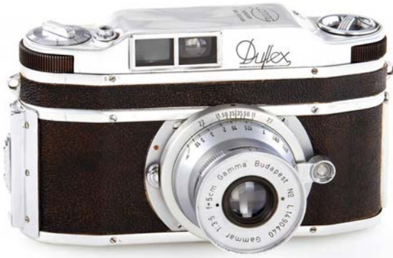
1. Duflex: The first camera with eyelevel viewing, made in Budapest in 1947 by inventor Jeno Dulovits. The camera was the first to have instant return mirror, bayonet lens mount, auto diaphragm closure before the exposure.
