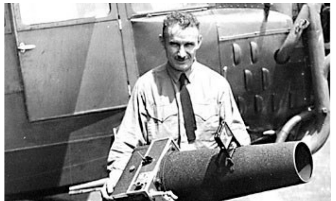
8. K-20 Aerial camera designed by Sherman Fairchild. He had numerous patents in this field to ensure film flatness across the film plane during exposure by an air suction mechanism from behind the film pressure plate.
