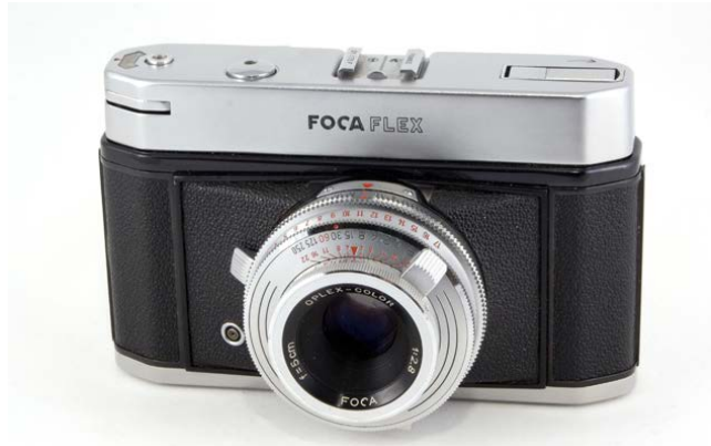
The mirror in Focaflex moves down, instead of up. This keeps the body very slim with a flat top.
