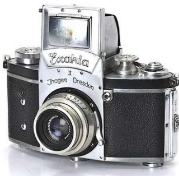
3. Kine Exakta from Dresden: The first commercially successful SLR, designed by Johan Steenberg from Netherlands (left), and Karl Nuchterlein (R). The camera featured a bayonet mount, focal plane shutter, lever advance film transport.
