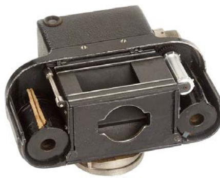
2. Sport: The first 35 mm SLR made in Russia in 1934, a year before Kine Exakta (designer unknown). It featured a reflex mirror that swung up, and a focal plane shutter that utilized single blades for the first, and second curtains.
