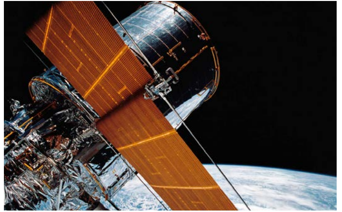
Above-left, an astronaut riding on the 15 meter canadian made robot arm to complete the installation of Hubble in space. Right, the solar pannels are shown in deployed position, fully extended out by Bistem tubes (see text for details).
