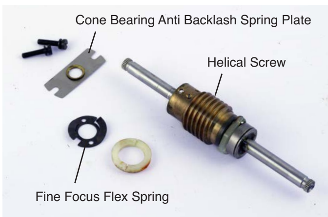
Fine Focus Bearing Assembly: Consists of a single ball bearing that rides against a rotary wedge shaped ramp.
