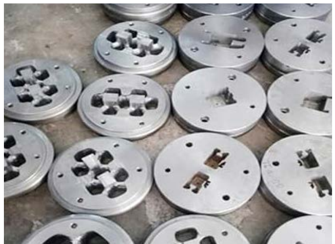
Optoform II: the lowest cost optical mount ever produced for prototyping. Right, extrusion dies for various profiles.
