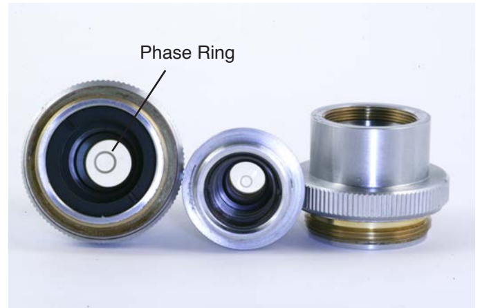
Phase contrast optics: Annular Diaphragm (left), and phase rings behind each microscope objective (right).
