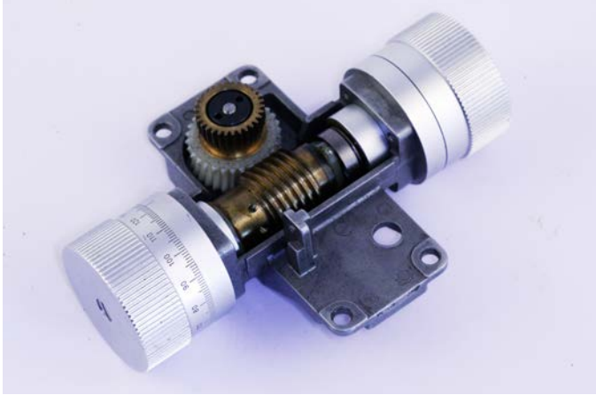
Fine and Course Focus assembly without the central fine focus knob in some of Leitz models introduced in 1970's.
