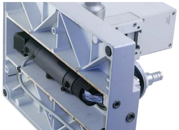
Relay prism assembly: The relay prism uses a pentaprism, and right angle prism for image transfer at the base (right).
