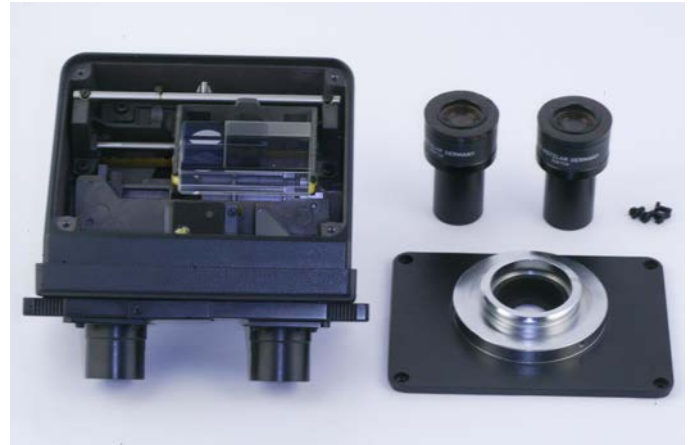
The trinocular head assembly: Belt driven 3-position beamsplitter translation for switching viewfinder/video light path.
