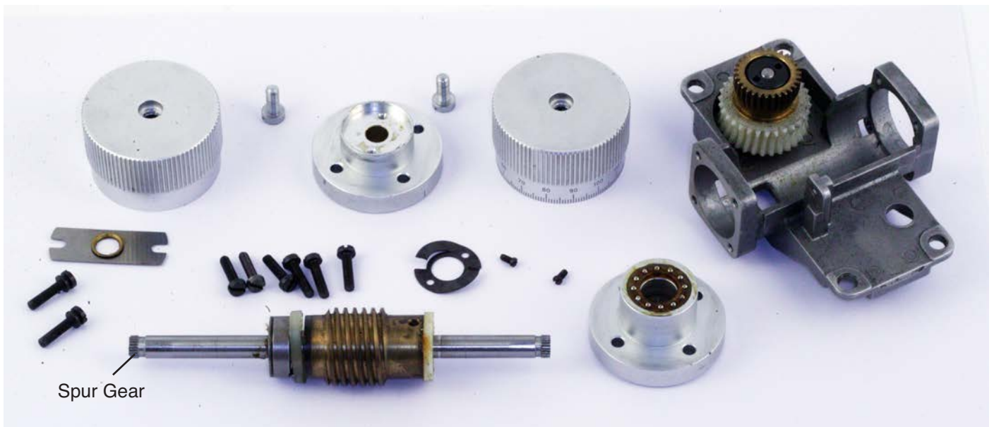
Fine and Course Focus components are reduced in this alternate design by combining them together.
