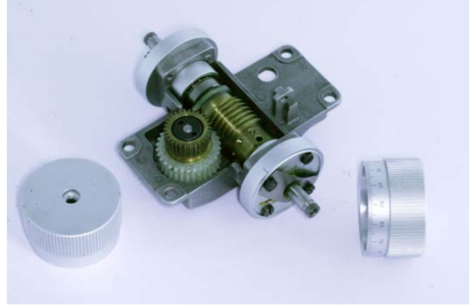
Fine and Course Focus assembly without the central fine focus knob in some of Leitz models introduced in 1970's.
