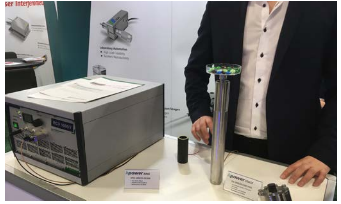
Piezosystems Jana , High precision, high load piezo actuator can micro-position up to 30 pounds in 100 micron range at high speed. One obvious application would be shock and vibration testing of opto-mechanical/electronics assemblies.
