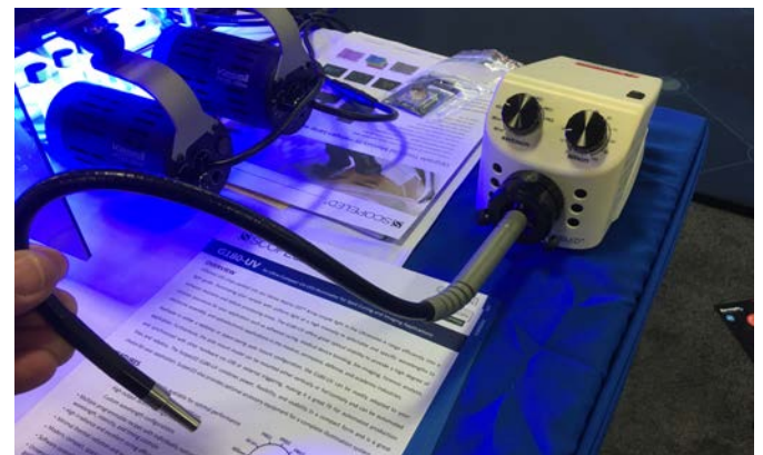
DiCon offers LED based fiber optics UV lamp illumination. Its wavelength adjuster is not a rotating filter wheel, but an electronic adjustment knob to adjust the LED output wavelength. The light guide is liquid filled.
