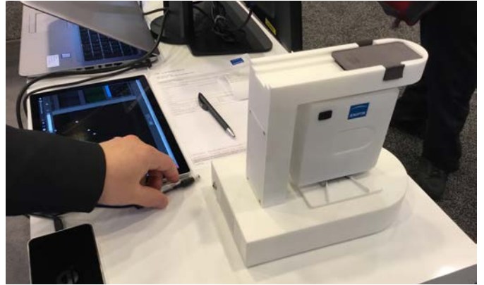
Compact scanning Inverted microscope by Jenoptik . The wireless controlled microscope (right), has detachable module mounts on a 25x25 mm scanning stage on the base, and the sample is held on removable (black) sample holder on top.
