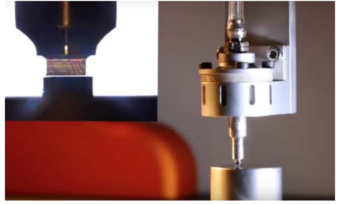
Touchless Automation has invented a machine that could lift and transport miniature components without touching them. This technology has active control of airflow to lift small parts, with sucking force dependent on weight, and size.
