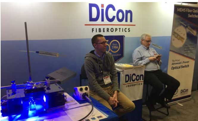
DiCon offers LED based fiber optics UV lamp illumination. Its wavelength adjuster is not a rotating filter wheel, but an electronic adjustment knob to adjust the LED output wavelength. The light guide is liquid filled.
