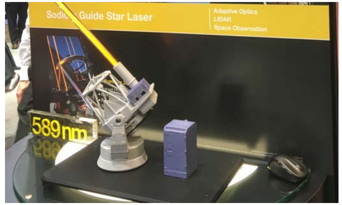
Toplica displayed 589 nm laser mounted on a telescope model that produces artificial star for deformable optics. Deformable optics is essential for telescopes above 25 cm in diameter to cancel out atmospheric turbulations.
