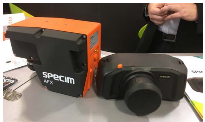
Spectral scan cameras (right), Specim has introduced a new airborne unit in addition to their previously announced handheld device. There is a scanning device inside that records multiplicity of images in the visible and IR range in 1 Sec.
