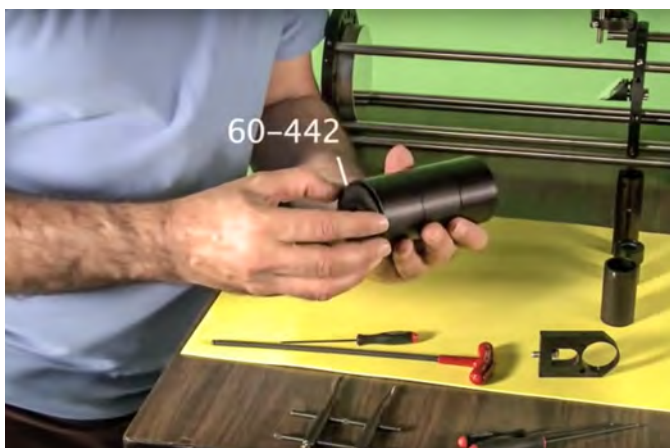
End plate 60-422 is added to one end
