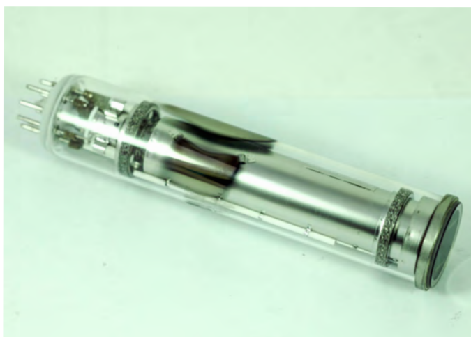
The Vidicon onboard Voyager spacecraft is based on the same television camera image readout scheme invented by Farnsworth in 1914. All the planetary images taken by Voyager that we still enjoy today has been taken by this 1.25" diameter device. Courtesy, OMiD museum.
