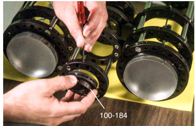
Side mounting of Minioptic 100 with Macroptic 150 via side connector 150-216.
