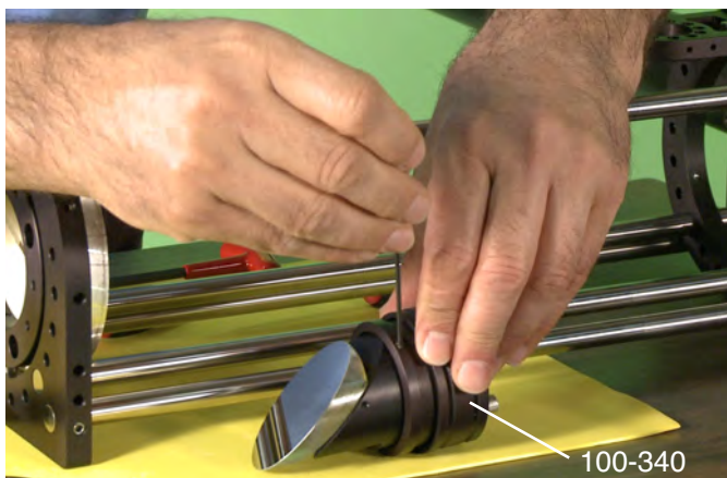
Stepping up Minioptic 100 accessories, i.e., 100-340 to fit inside Macroptic 150 mounts via centering ring 150-160. Mirror mount 100-342 has a threaded hole pattern for direct mounting to Microptic 50 mounts such as 50-100/50-104.
