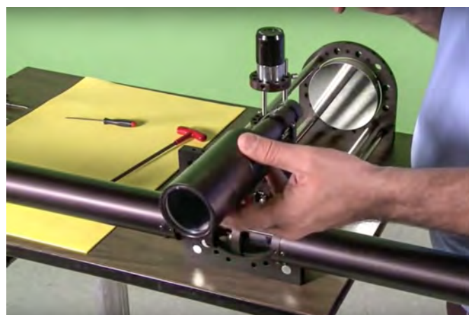
The finder scope is inserted into the mounting column
