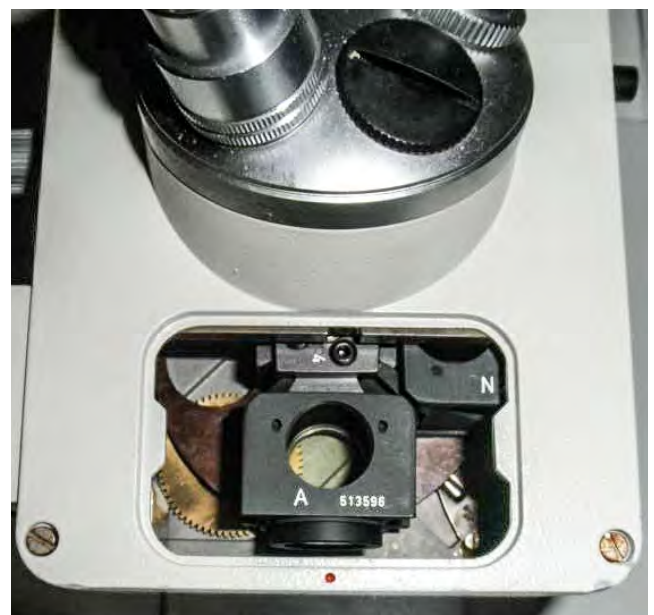
Leica Diavert inverted microscope with mercury light source for fluorescence microscopy, and Halogen lamp source for phase contrast observation. A close-up of the beamsplitter turret for beamsplitter cubes is shown on below, right.
