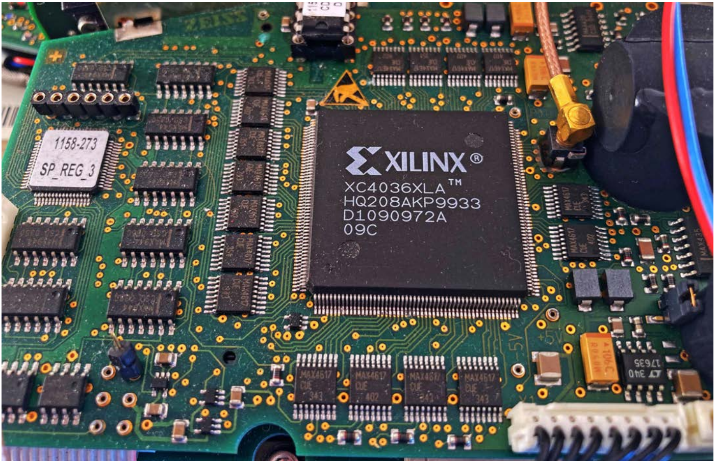
XILINX 4036 XLA processor chip on board 9 handles the signals from META detector.
