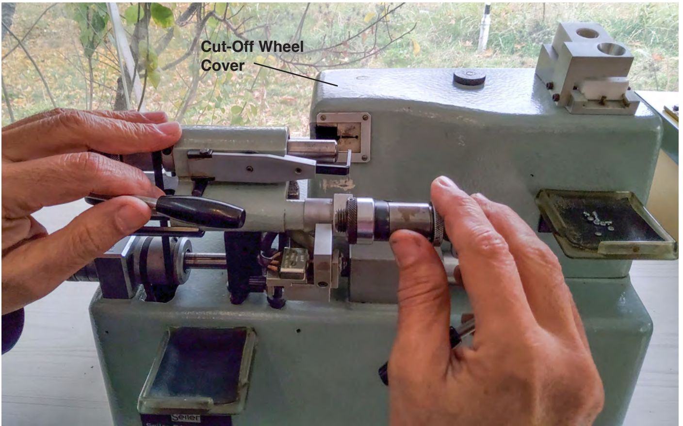
Cutting off the setting stem to length, and installing the crown is done precisely with this machine.
