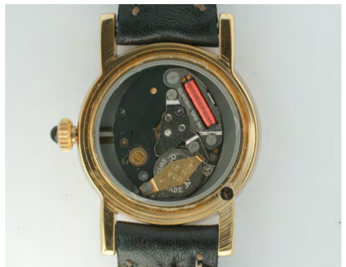
A ladies watch, product of Zimak watch factory (left). The back cover is removed for battery replacement (right).
