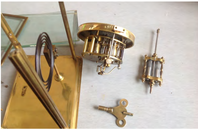
Repairing a French made Woslon & Powel clock
