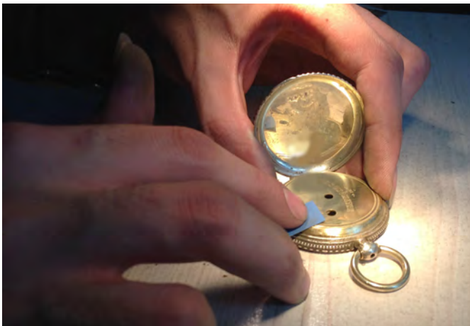
Hand polishing the case of a pocket watch
