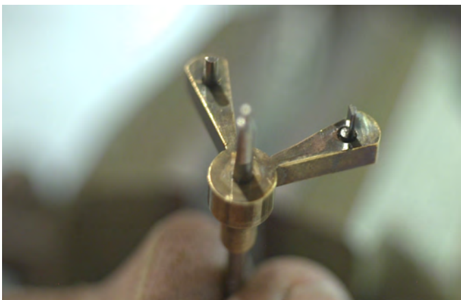
One of the pallet pins needed replacement
