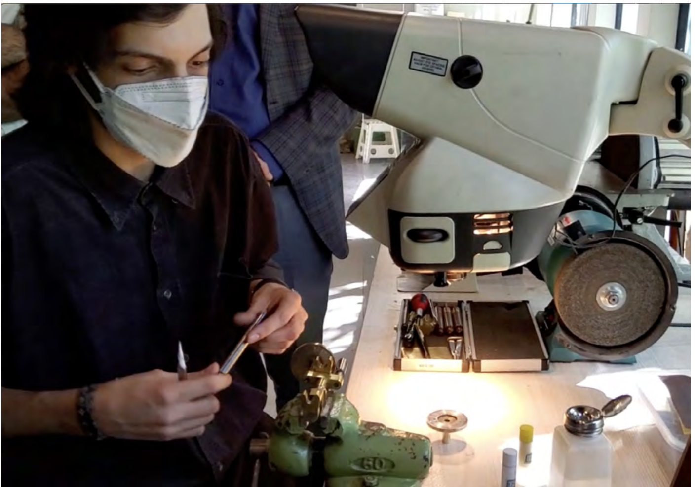
Men's watch with mechanical movement, and Farsi numerals with Zimak's logo, stainless back, and leather straps. Below, the polishing department uses polishing tools such as Lorch to polish various watch components before plating.
