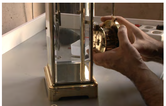
Reinstalling the movement on the main housing
