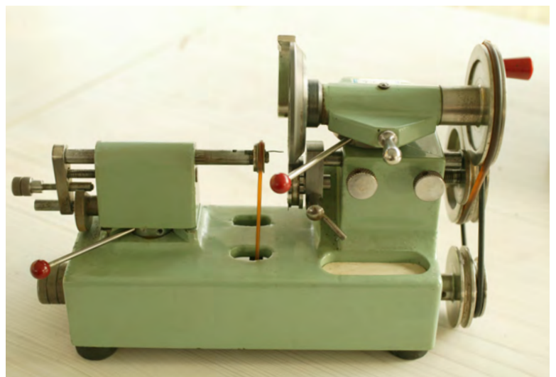
Pivot polishing the balance wheel of a pocket watch
