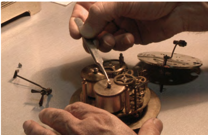
Removing the spring box for cleaning and lubrication
