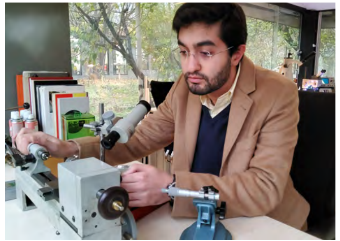
Watch case modifications on Levine lathe
