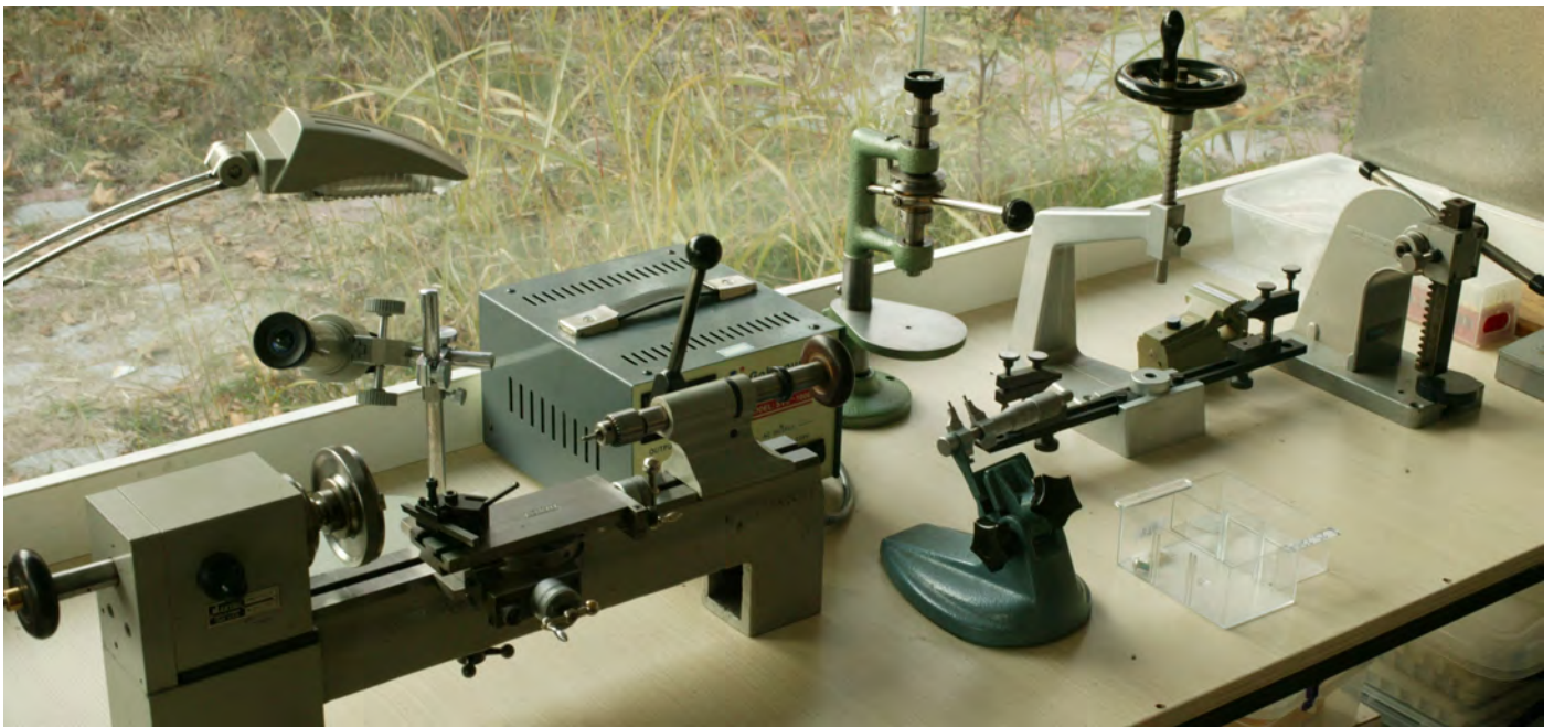
Levin 10 mm precision lathe, Bolova microscope, Bergeon drill, Bergeon tapping and boring stand, and precision press.
