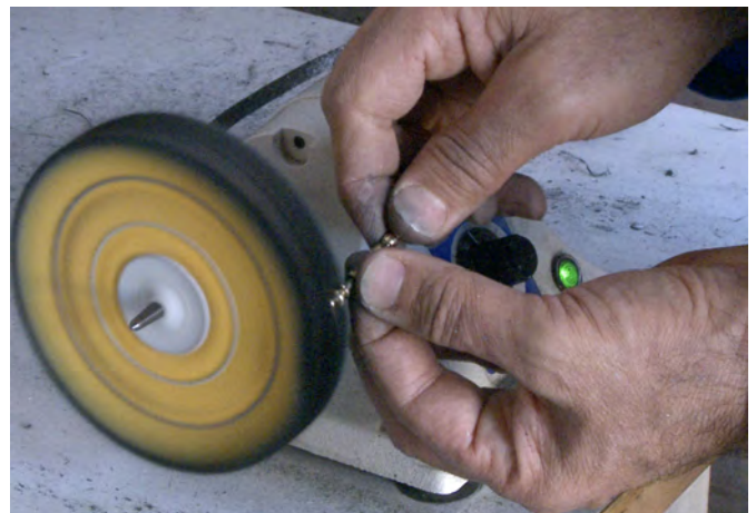
Hand polishing the Woslon & Powel Pendulum
