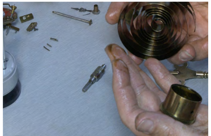
Remake of one of the broken spring hooks
