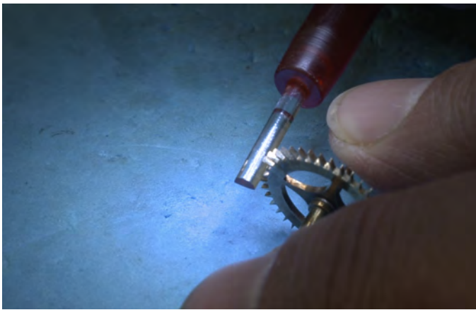
Fine polishing the pallet wheel with a sapphire file
