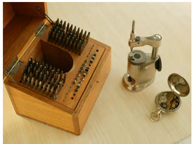
Tightening the mounting bore of a watch hand by punching
