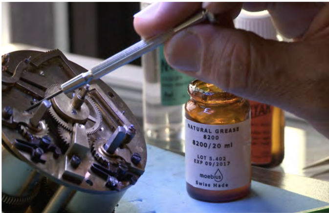
Appropriate lubes are applied to all moving parts
