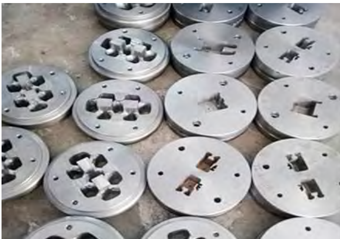
Left, extrusion dies for various profiles. Right, gradual formation of 20/20 Aluminum extrusion profile through dies.
