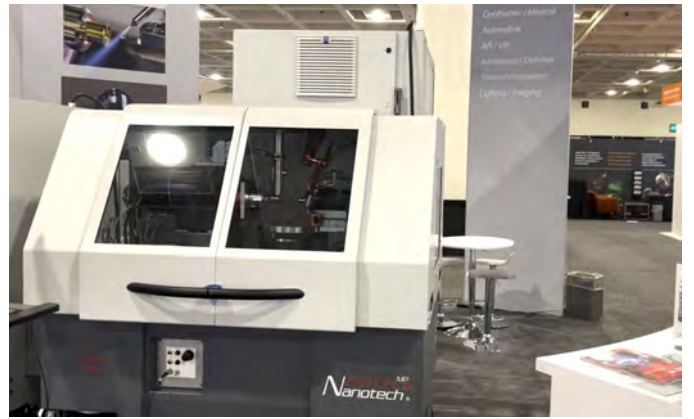
Nanotech precision diamond turning machine (right). Inside the machine is shown with chuck, Aluminum chip vacuum, and cutting tool.
