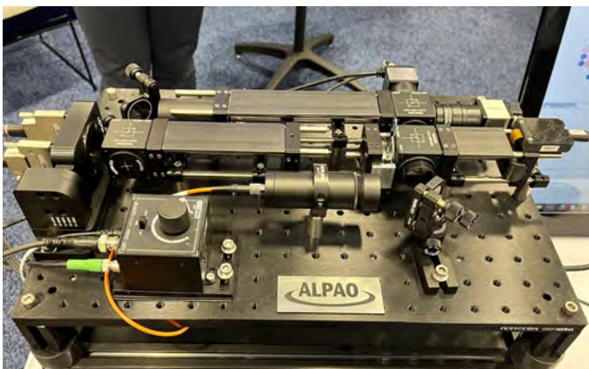
ALPAO France, deformable, or adaptive optics is displayed in this small breadboard setup built with cage system.
