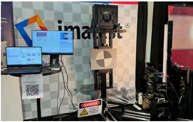
Ground level Image tester by imagtest performs MTF testing of lenses with motorized optical rail.
