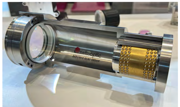
This huge linear bearing guide rail (right) always catches the eye at shows with their slick design, by Swissoptic
