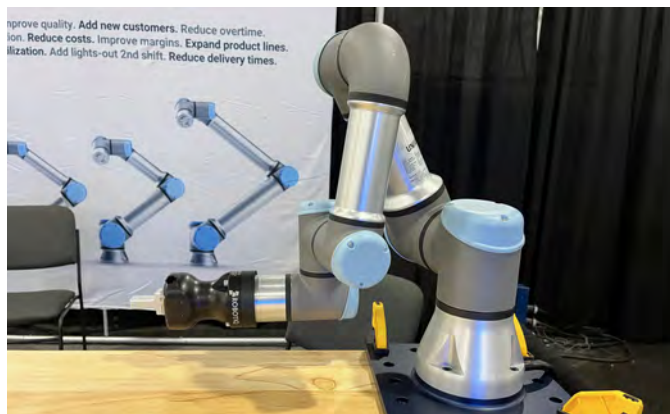
Robotic arm at 3D Infotech booth with AI camera head for distance, and object recognition performed programmed tasks.
