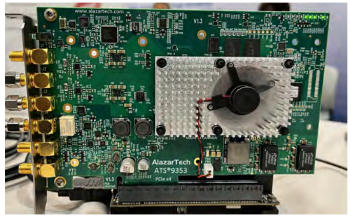
Signal digitizer boards by AlazarTech for high speed multichannel signal capture, and play back. www.alazartech.com
