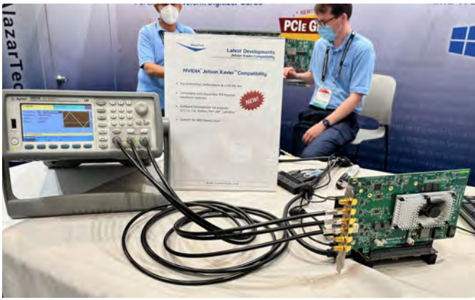
Signal digitizer boards by AlazarTech for high speed multichannel signal capture, and play back. www.alazartech.com
