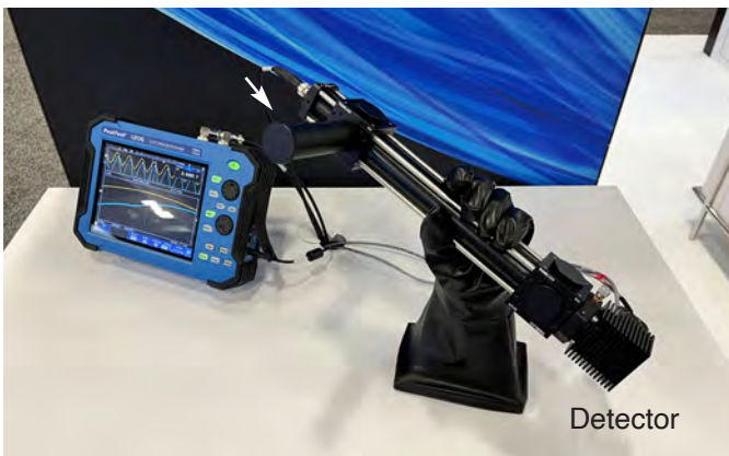
Co2 gas detector using detector made by NanoPlus. The Co2 gas enters through the tube (arrow)
