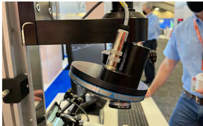
Close up of the Trioptics machine reveals motorized nose turret, and control/measurement software.
