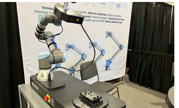
Robotic arm at 3D Infotech booth with AI camera head for distance, and object recognition performed programmed tasks.
