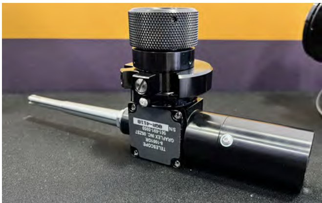
The rifle scope alignment tool is inserted on the barrel, and projects a laser beam for the scope's alignment (Salvo).
