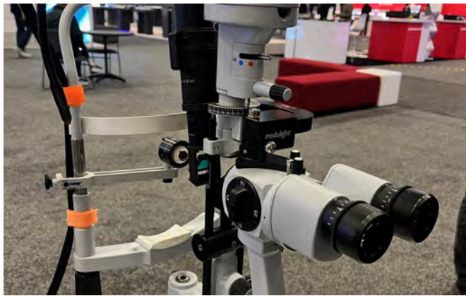
Slit lamp attachment for eye surgery by Modulight may be attached to slit lamp by various manufacturers. Right, computer interface.
