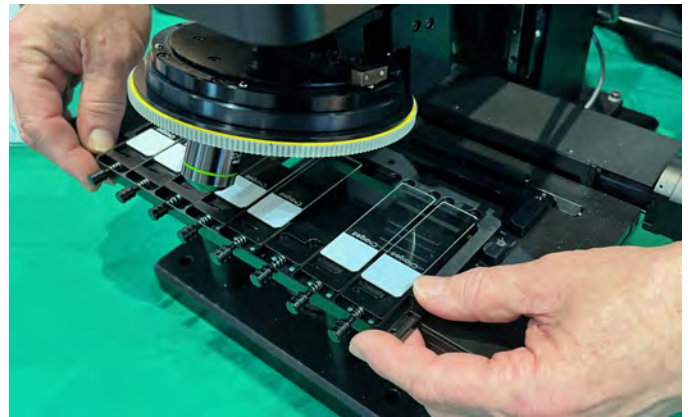
Prior's multi slide carrier (above, left), and how it's designed to be easily interchangeable.
