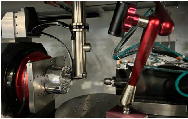
Nanotech precision diamond turning machine (right). Inside the machine is shown with chuck, Aluminum chip vacuum, and cutting tool.
