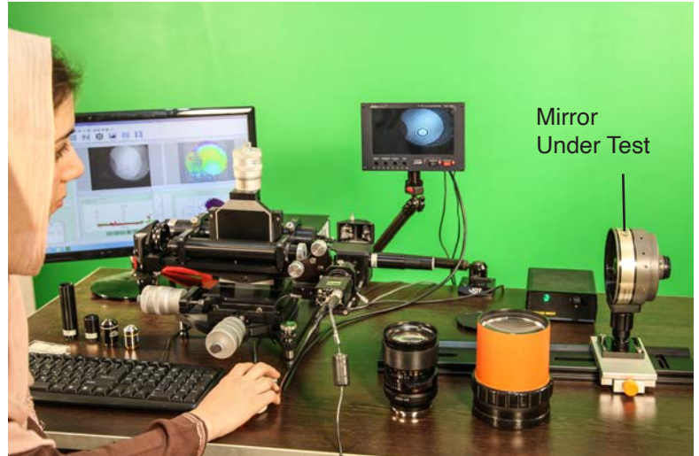
Above, Buccini Interferometer. Right, using the interferometer to measure the surface accuracy of Celestron C90 spherical mirror.
