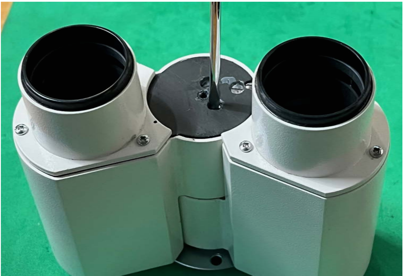
Prism adjustment screw has a very short range: It fine adjusts the vertical error of image overlap between eyepieces.
