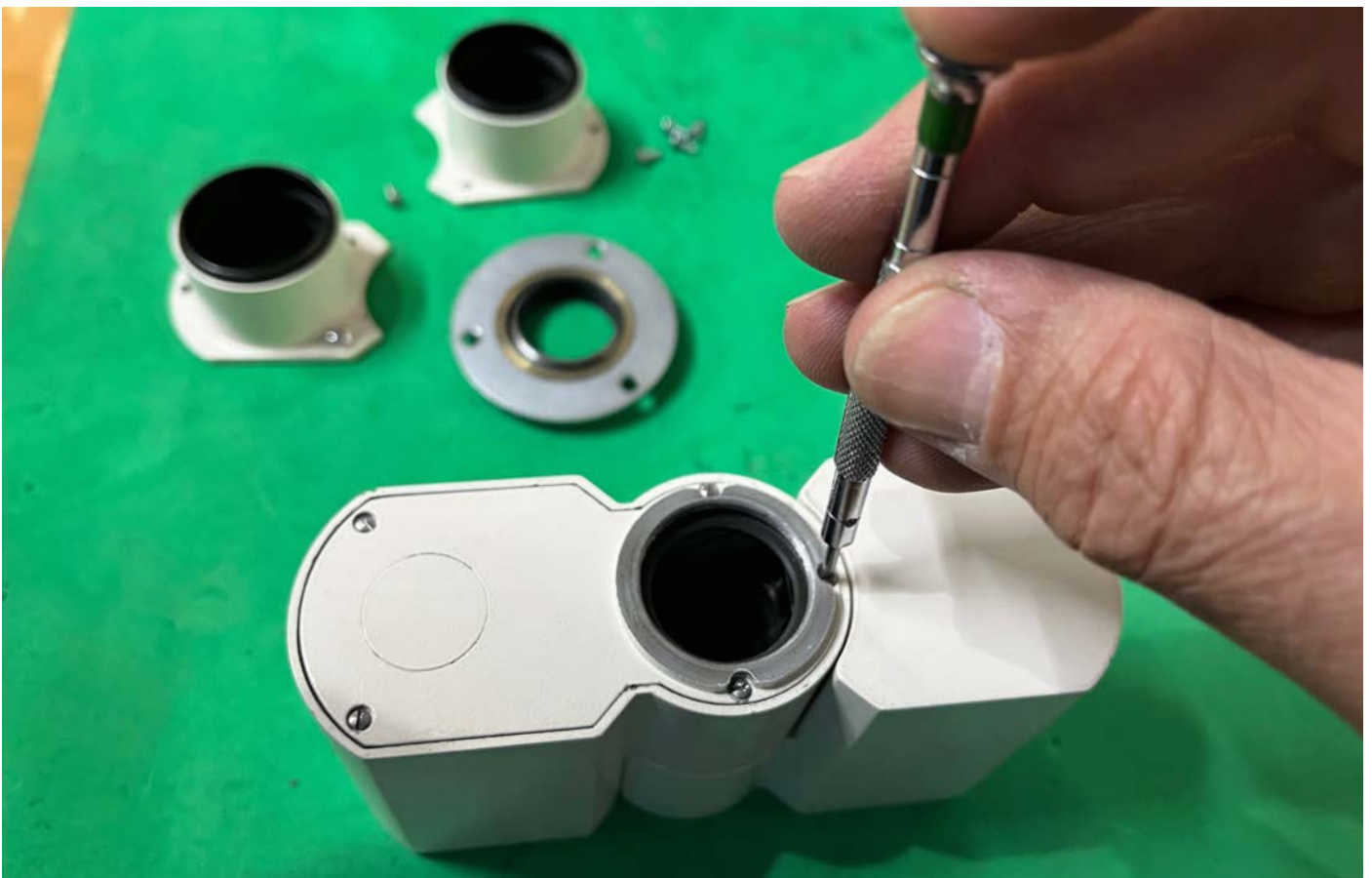
Reassembling the binocular head.
