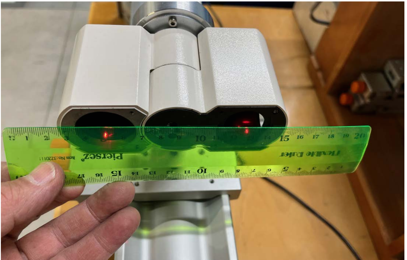
Eye distance measured at binocular head.
