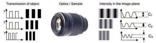
Test target (left), and its image by the lens (right)
