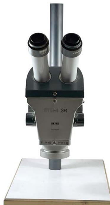
1980's Zeiss Stemi Stereo Microscope with 60 degrees inclined viewing, and LED light illumination
