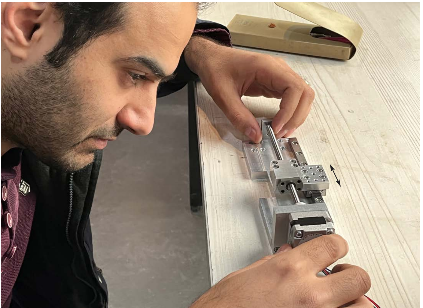
Aligning the ball screw with the linear bearings axis.
