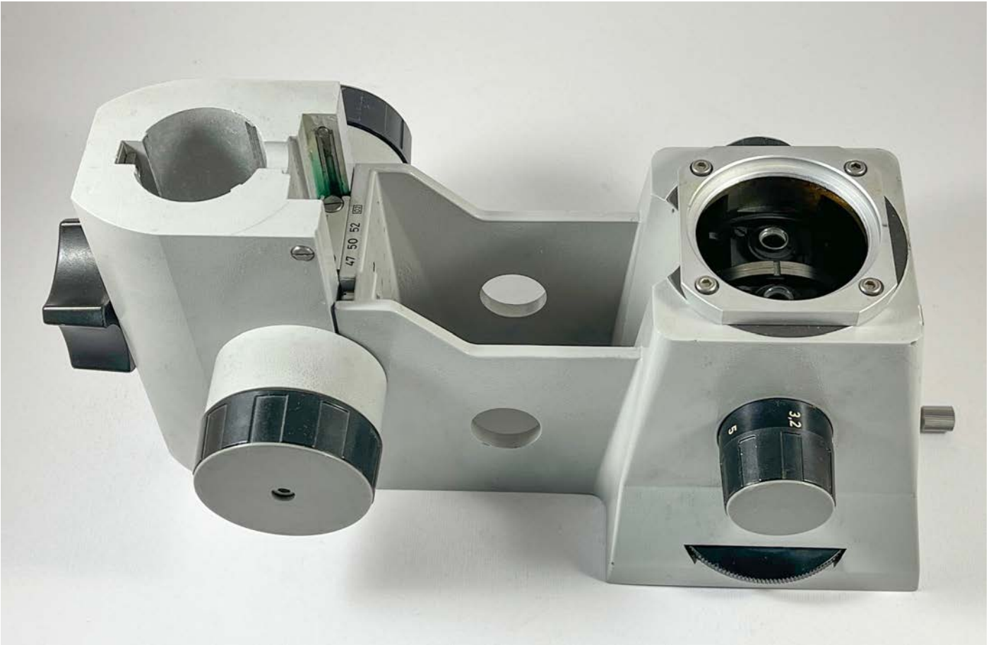
Bottom view of binocular optics with focusing knob, and magnification change.
