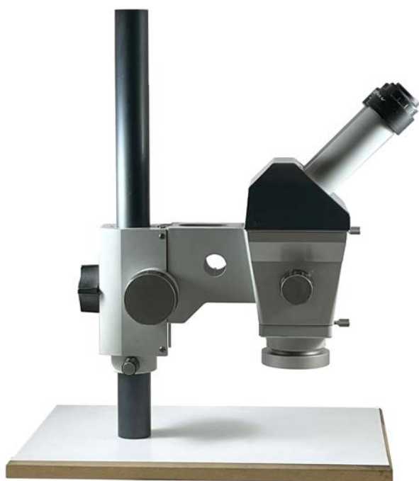
1980's Zeiss Stemi Stereo Microscope with 60 degrees inclined viewing, and LED light illumination
