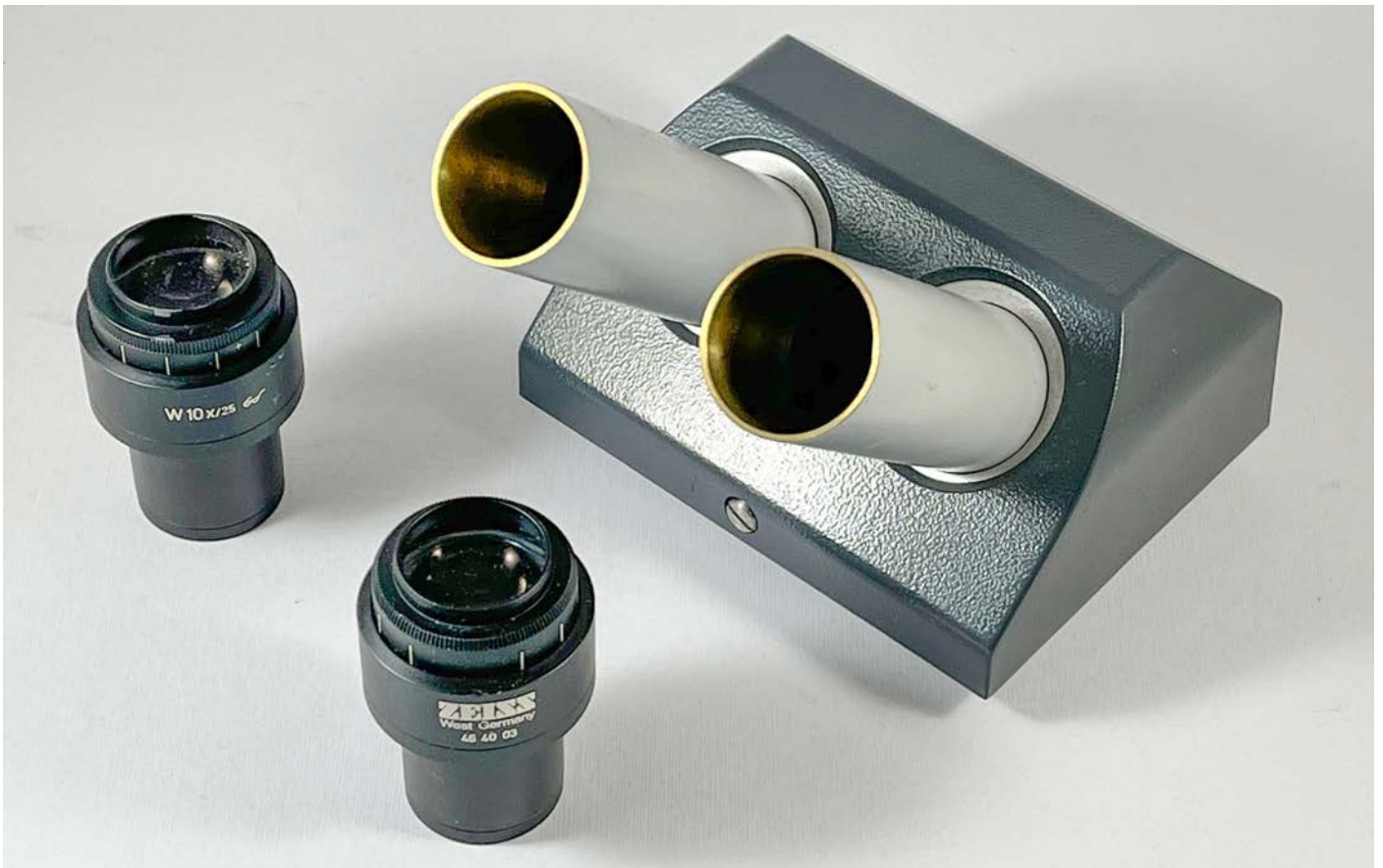
The binocular head removed to show its two slanted eyepiece tubes.
