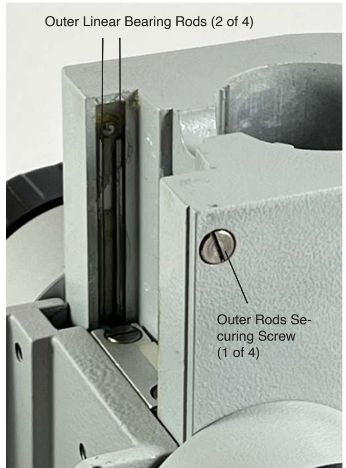
Linear travel of focusing mechanism utilizes steel rods as guide rails for its linear bearing path way.
