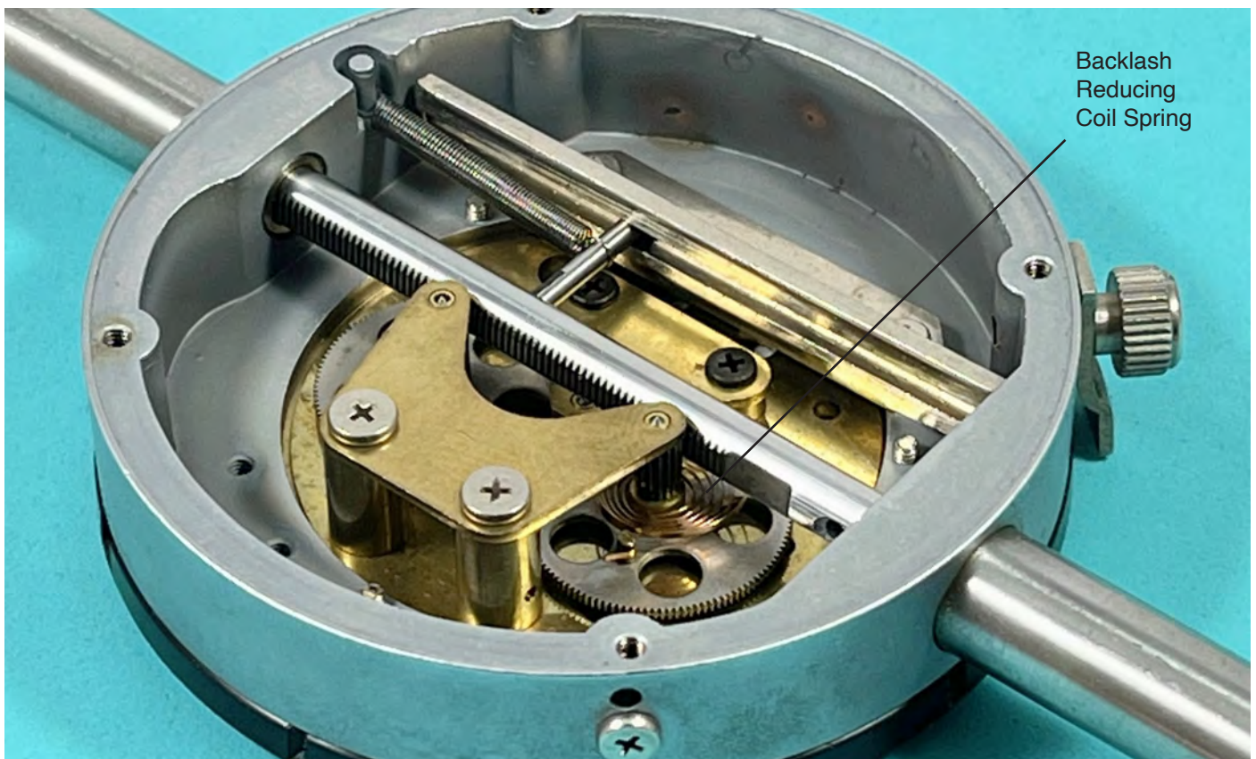
0.01 mm pointer shaft is driven by gear C, which is behind the mech plate. Concentric 1 mm pointer is driven by gear A as shown above the mech plate, and gear B (see Page 7).
