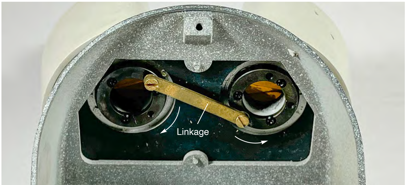
The viewfinder assembly shows the cemented image correction prism pair taken off for the left eye.
