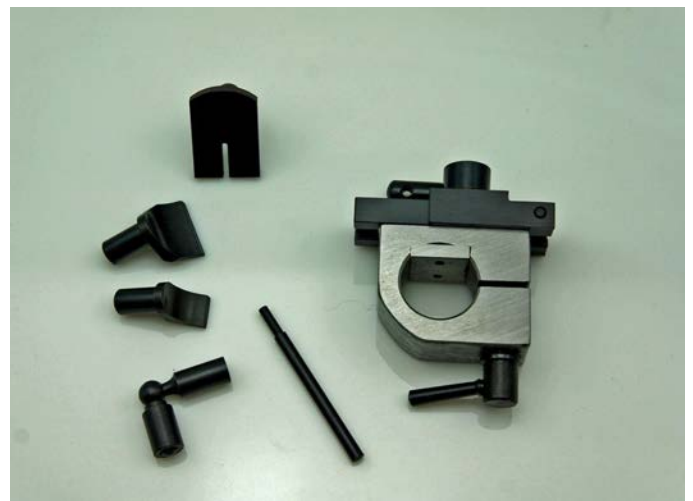
Traditional watchmaking lathe bed (still manufactured by French, Bergeon) resembles the A-Line system by Newport. Newport utilized the same mounting scheme utilizing a set screw to both align, and secure their mounts.
