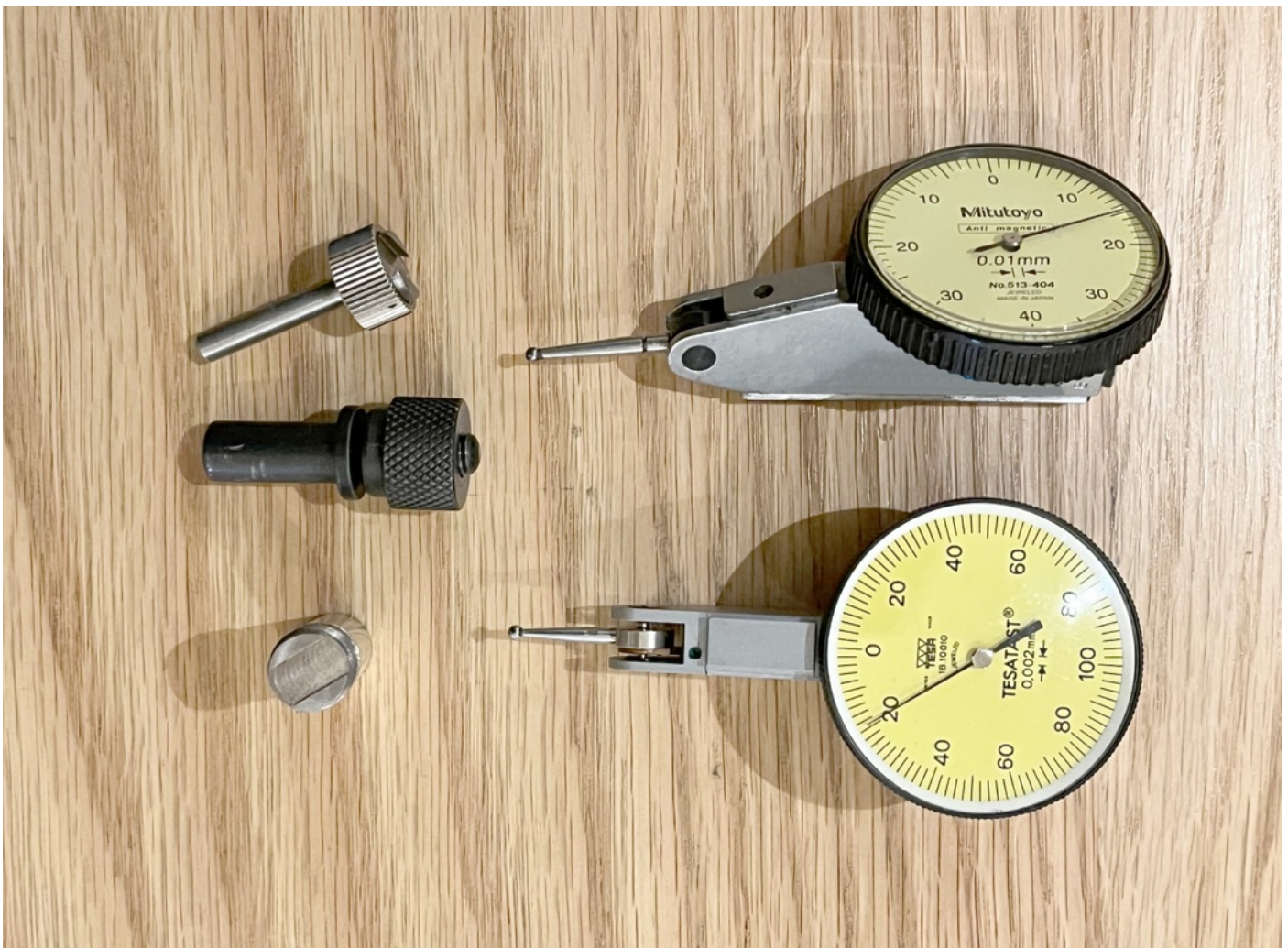
Mitutoyo dial indicator with 0.01 mm resolution (above), and 0.002 mm resolution (below).
