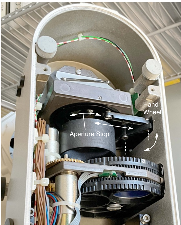
Above, the most clever design I have seen in iris diaphragm control, basically linking two dials by utilizing a lever.
