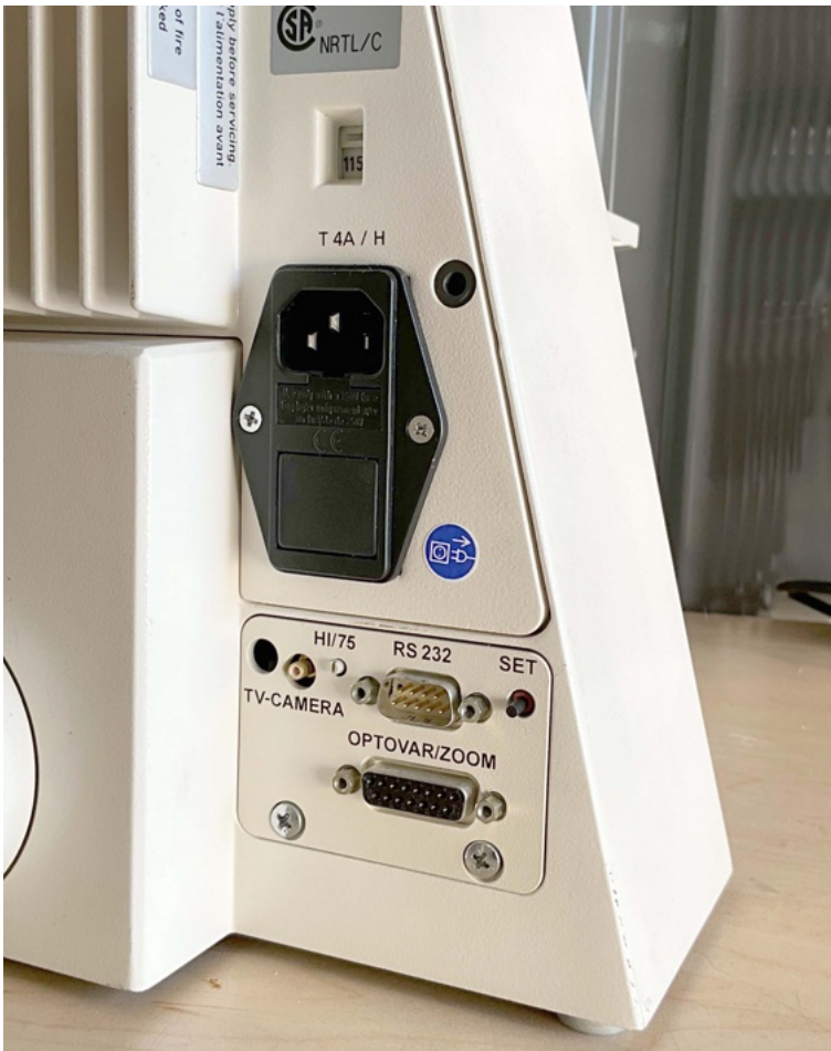
Back View, with power input, and Computer serial interface
