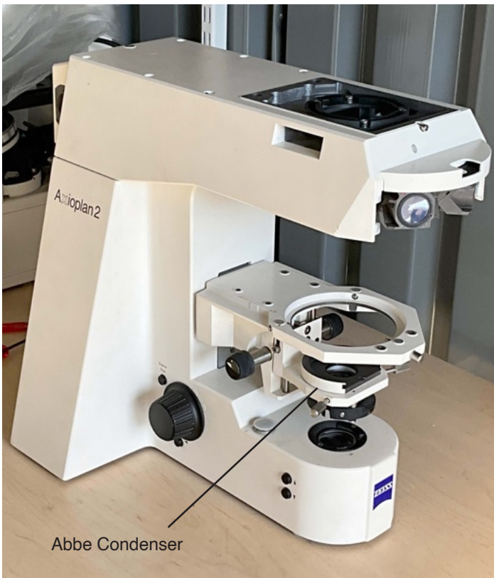
Sample stage removed to reveal focusable Abbe Condenser
