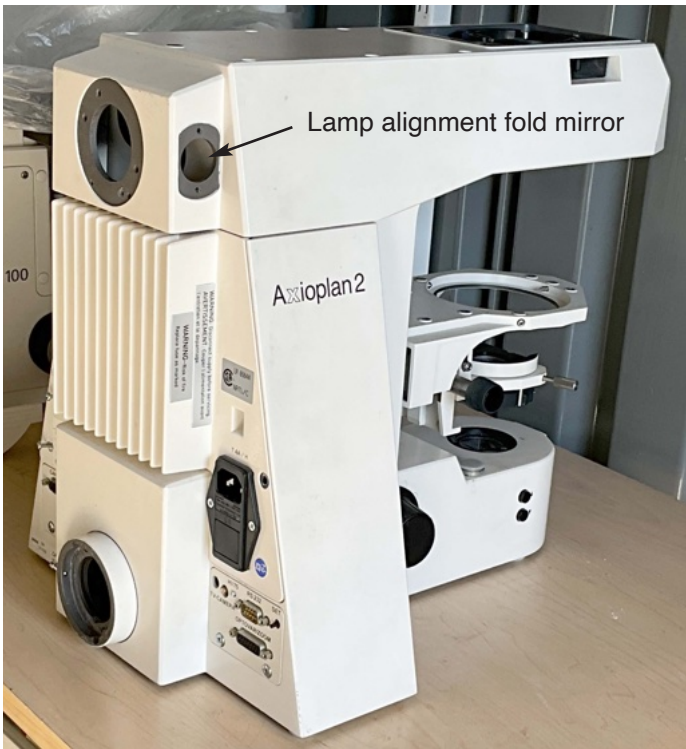
Beginning disassembly: Lamp mount, and reflector below
