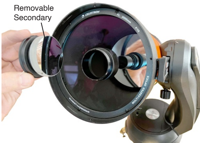
Removable secondary mirror allows mounting SLR cameras at the focal plane of the primary mirror.
