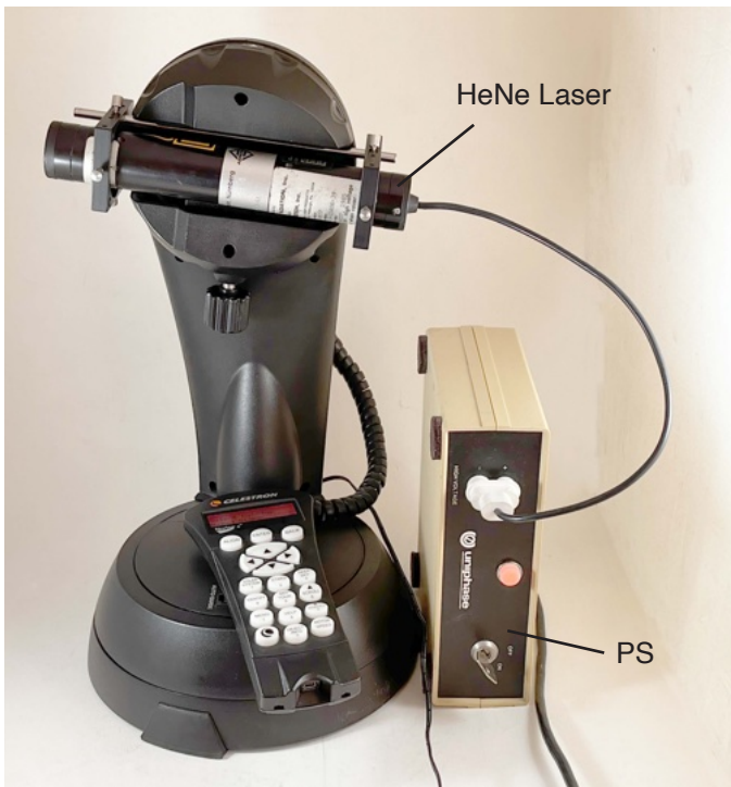
Mounting a HeNe laser in place of the telescope (left) to measure its backlash: By turning the encoder behind the motors in one direction, and then in reverse direction, the backlash is measured to be 2.5 turns. Celestron compensates for this by always passing a point of interest by a few degrees, then returning to the intended point to compensate for backlash.
