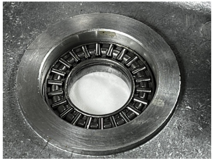
Drive motor (left), and close up view of roller bearing at the center of horizontal axis (right ascension). This type of roller bearing is utilized where heavy loads are to be supported by a compact, and relatively maintenance free design. Celestron supports it by a hardened flat washer on top, and three Teflon bushings on the bottom (see P16).
