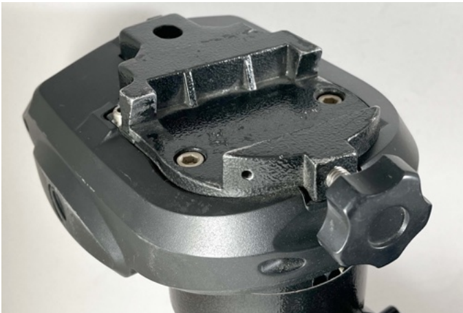
The dovetail mount (left), and north-pole alignment knobs (right). There is a connecting cable called: "Dec Port", that connects the right ascension drive motor with the main electronics control box (right).
