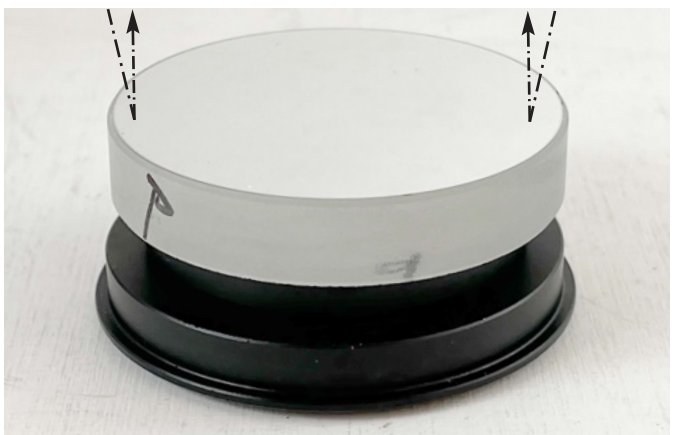
The secondary mirror is mounted on a tilt platform. Alignment pin ensures correct orientation of mirror to preserve its alignment with primary mirror.
