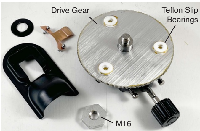
Declination (Altitude) 240-tooth gear (left) with Teflon slip bearings. Celestron utilizes a large diameter cardboard washer behind the slip ring. This material is apparently utilized to produce constant friction. The Altitude axis can be manually rotated by hand.
