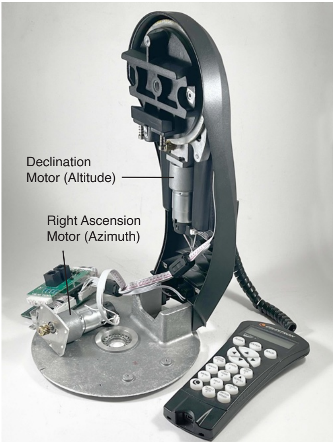
Declination, and right ascension rotary axis drive motors (left) are controlled by electronics board, and key pad. Both axis utilize roller bearings and Teflon pads to deliver smooth rotary performance.
