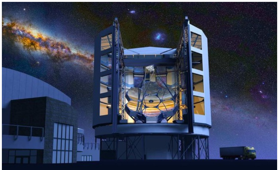
Giant Magellan Telescope has a 25.4 meter aperture. It is expected to have a resolving power approximately 4-10 times greater than the Hubble Space Telescope and four times greater than the James Webb Space Telescope. However, it will not be able to observe in the same infrared frequencies as space-based telescopes.
