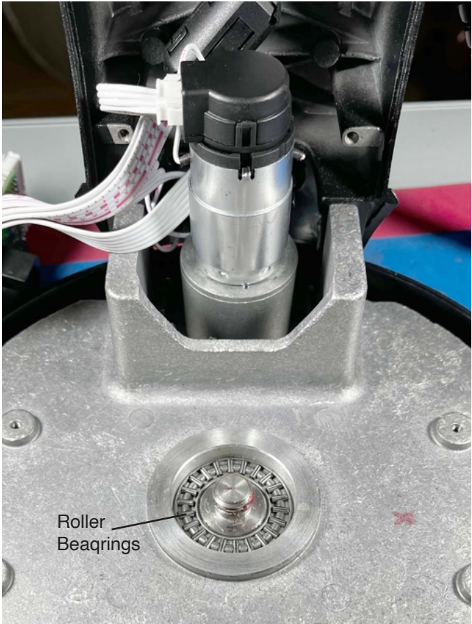
Declination, and right ascension rotary axis drive motors (left) are controlled by electronics board, and key pad. Both axis utilize roller bearings and Teflon pads to deliver smooth rotary performance.
