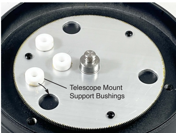
The entire weight of L-Shaped telescope mount (right) rides on three Teflon support bushings (left). This design avoids heavy/expensive bearings that large telescopes use. The large central 519-teeth gear fits in between three Teflon bushings (left) to provide a smooth — wobble free rotation. The gear ratio of this large gear to motor's drive gear is 1:28.8
