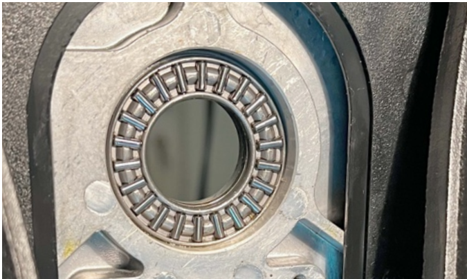
The roller bearings of declination axis (left), and is fully assembled, and secured by Aluminum tension nut (right).
