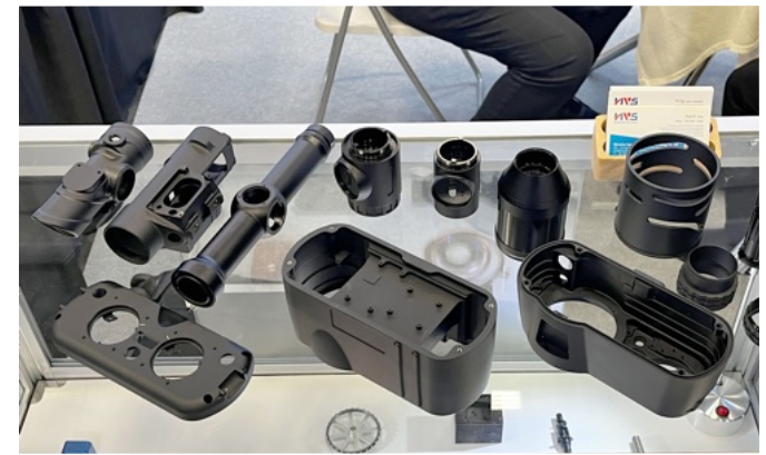
25. These beautiful CNC work by Honvision (right) is a disassembled night vision unit that fits together as if it's injection molded plastics. The anodized finish was so soft, it felt like rubber coated metal. The Chinese have come a long way.
