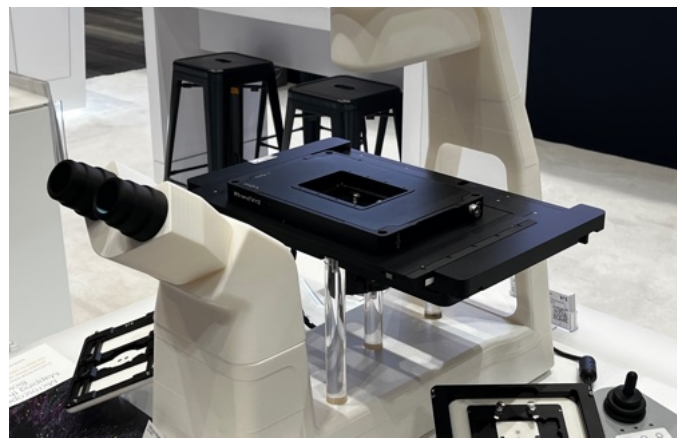
2. Zaber builds translation stages for microscopy, and fine focus stages (below, right). On display was their modular platform for automated Fluorescence microscopy (left). One of my favorite designs is this tilt platform utilizing C-flex bearings
