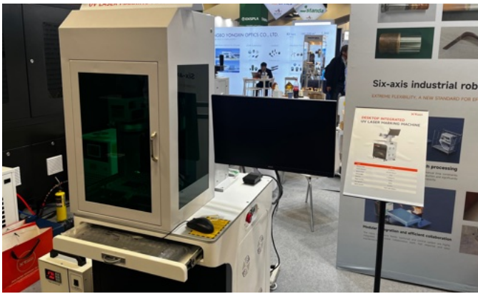
50. XT Laser's desktop enclosed UV laser marking machine with floor standing laser source. Side view of the machine shows height adjustment knob to accommodate various sample heights.
