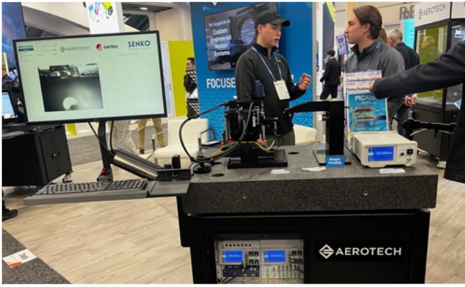
47. This silicon photonics setup at Aerotech booth is for aligning fibers with a photonics chip. The special patch cord consists of eight fibers that are aligned with an identical number of interface spots on the chip. The probe arm is held by
