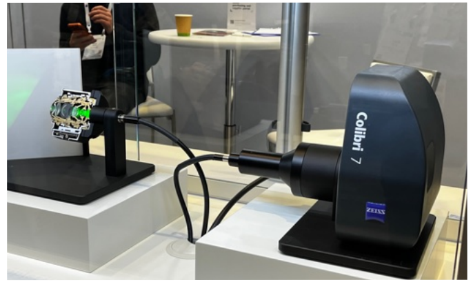
12. This biomedical imaging lens Zeiss was so beautifully sectioned, it made the cover of current issue of Optomechanix. On the right is a multispectral LED light source, and the close up picture of the left is a motorized microscope objective
