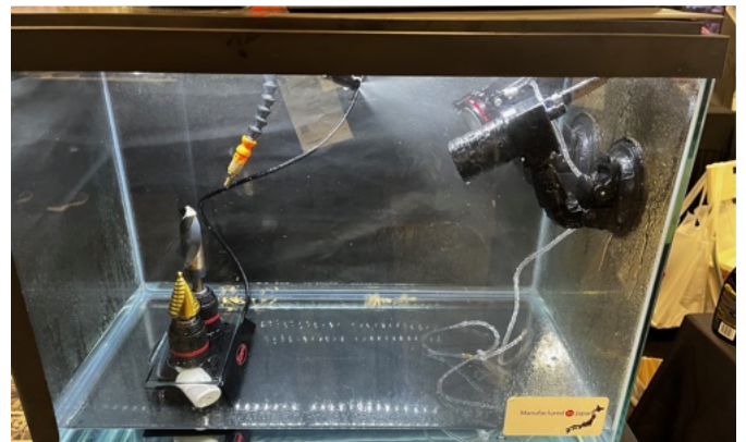
38. Cowa, the Japanese lens manufacturer displayed their harsh environment imaging lenses. The water proof lenses can be installed inside CNC machines (above) to show live view of the machining operation. A spinning front lens element
