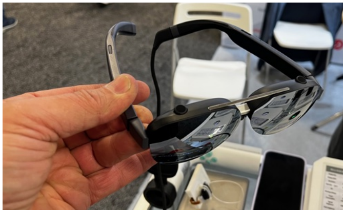
36. Rear projection eyeglasses by Rayvision Technology projects a high-resolution image above its field of view (right) at a 3m distance. See the vision section for a full range of these display glasses.
