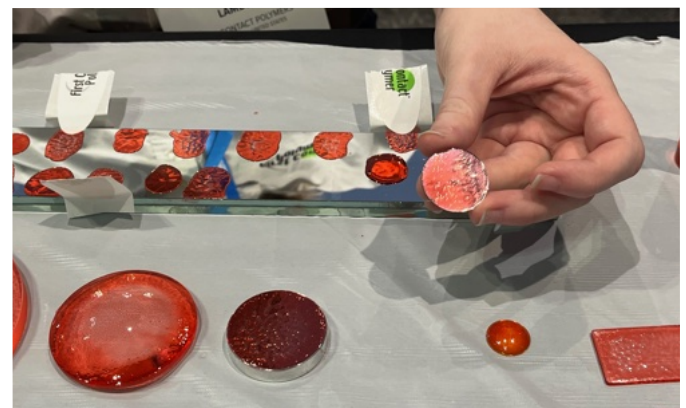
14. Photoniccleaning offers this chemical when paint sprayed on an optical surface, it dries to provide a protection coating, and it acts as a cleaning agent when peeled off.
