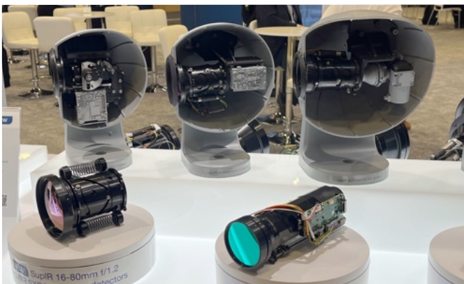
drones with domed optics. I would rather devote my talent to biomedical, microscopy, and astronomical applications. But just to show you how they fit the zoom lens, and image sensor inside the domes, they fold the light path (above, right).
