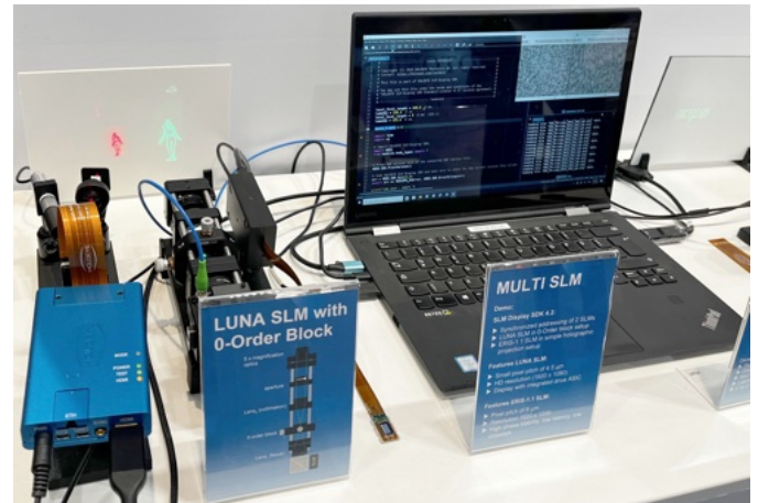
3. Holoeye provides SLM devices for various optics applications such as pattern recognition, etc. Each high resolution SLM is driven by a flex cable, and driver box (right). The signal is fed to SLM by a computer via USB cabling.
