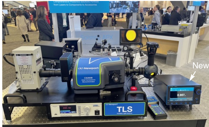
filter wheel (on the left). The power supplies are placed below the mounting plate with support legs, and carrying handles. The power meter is new according to their now subsidiary, Newport. There is a spaghetti of cables that are hidden behind
