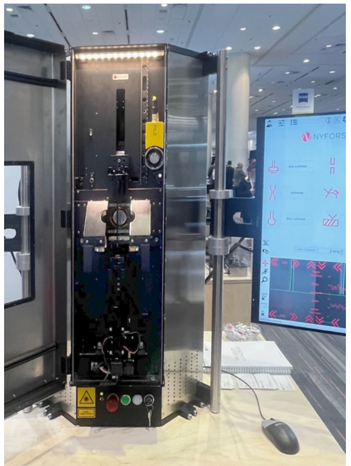
11. Nyfors displayed this fiber processing (Cleaving, linear splicing, end capping, inspection, etc.) system. The enclosure is ideal for cage system/Optoform instrument. Nyfors displayed this fiber processing (Cleaving, linear splicing, end
