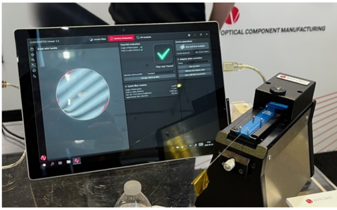
Fiber end inspection interferometer (Cleavemeter) for checking end surfaces of polished/cleaved fibers. The fiber end is simply clamped by a spring levered chuck, magnified by internal optics, and video camera.
