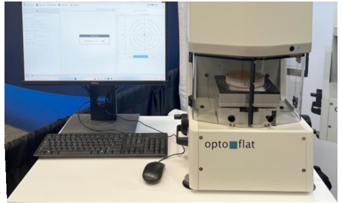
40. This downlooking interferometer by InterOptics measures surface flatness of plane optics. The fully enclosed housing effectively eliminates the effects of air turbulence.
