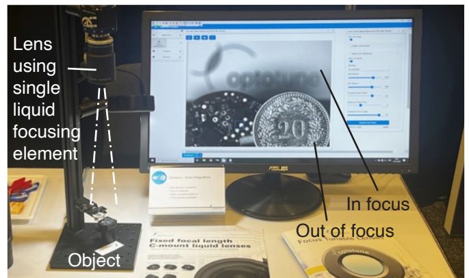
59. Liquid lens by Optotune (left) allows super fast change of focus, can be designed as part of a lens group (above).
