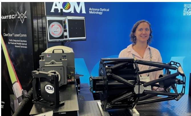
42. Arizona Optical Metrology offers a holographic mask for critical alignment of telescope's primary, and secondary mirror through interferometry. The system utilizes a Zygo interferometer, alignment mask, and accompanying software.
