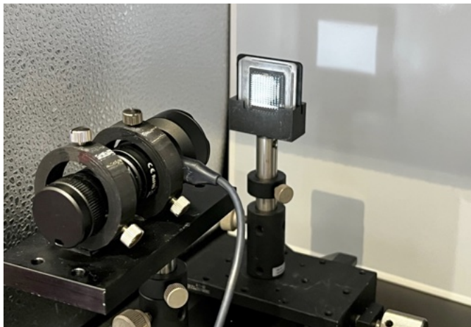
17. Isuzu glass company (Osaka Japan), makes these highly efficient diffusers that provide high transmission with uniform flat-field lighting at the object plane, i.e., projection LCD's or other critical illumination applications.
