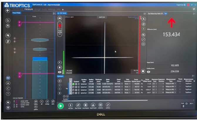
59. Trioptics lens measurement stand, and accompanying software checks lens/barrel centration, etc.
