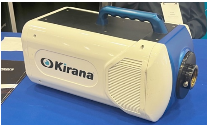
60. Kirana high speed camera in Specialized Imaging booth, is capable of capturing 1 million frames per second. Multi-spectral imaging indicates a built-in AOTF (acousto-optic tunable filter).
