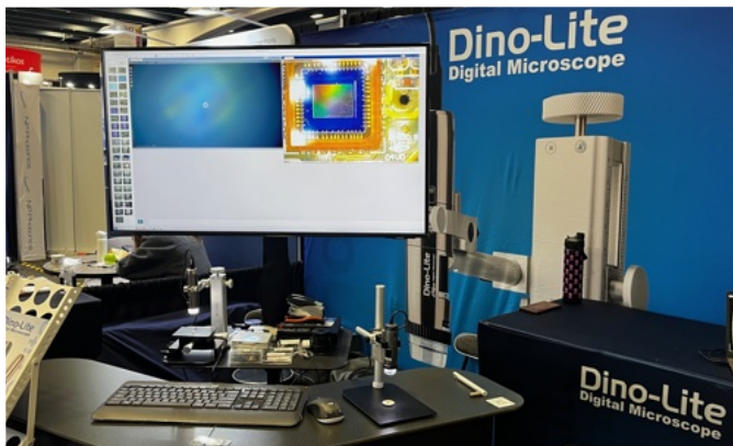
44. Dino-lite offers these modular stands, and accessories to build your own custom digital microscope setups. The compact stands allow precise X-Y-Z alignment of the digital camera, for image focus, and object centering at high mag.
