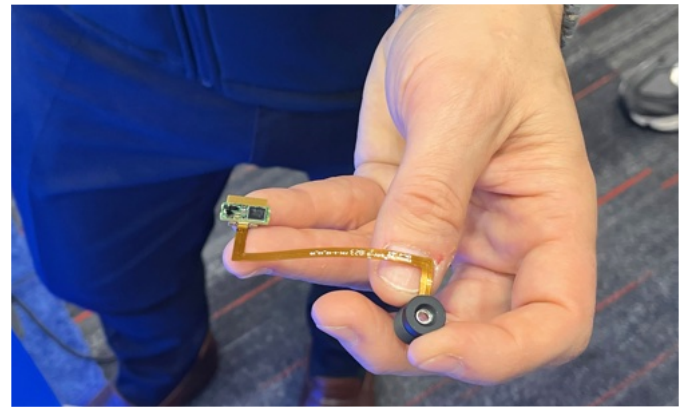
6. Corning Varioptic liquid lenses on display at their booth. Depending on the voltage applied, the lens could be divergent, flat or convergent. It's called electrovetting, and each lens acts as a capacitor. Visible transmission is near 100%. Corning offers both as single element, and imaging lenses.
