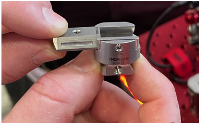
A lock screw rides inside a groove (left) that permits a limited travel without allowing it to come off. The spring-loaded tip of the screw would create a smooth sliding affect. It can also accept a positioning screw for fine vertical adjustment.
