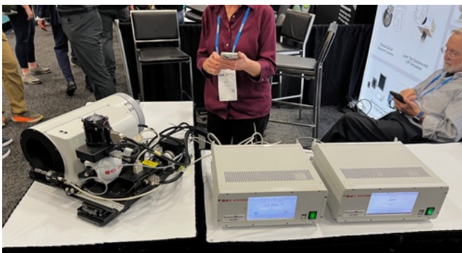
mirror, then a small mirror is cut out off from their side to maintain a high surface accuracy. The illumination source consists of an integrating sphere & filter wheel. The image sensor is positioned in front of the unit utilizing a pick off mirror.
