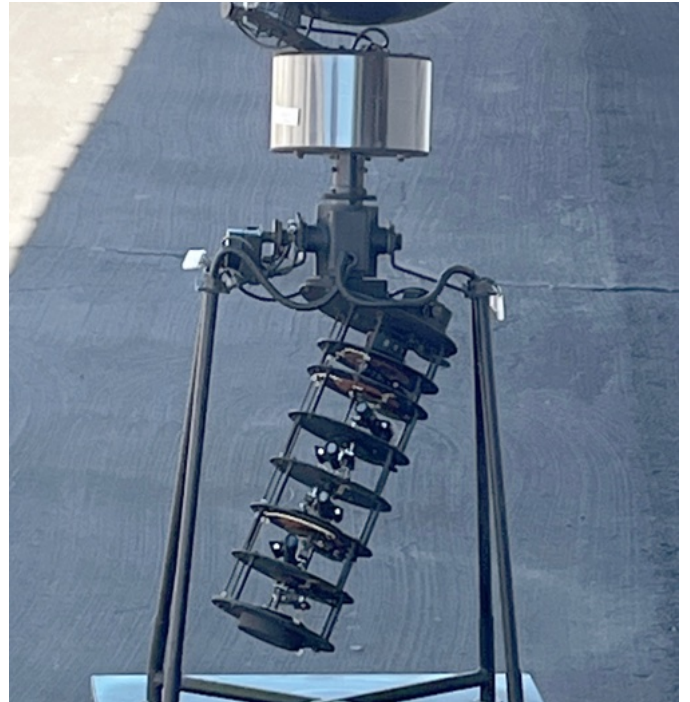
The electrical wiring of planetariums are challenging because it should be able to rotate 360 degrees on each axis. Some contacts like the central filament are powered by a brush + conductive disk method, similar to electric motor armatures.
