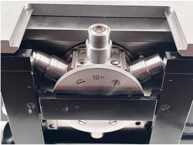
The objective turret in Zeiss Micro interferometer (left), and its focus indicator (right) has two sets of objectives. A set of three Linnik objectives, each useful for different magnifications. Intungsten light mode, it allows normal sample focusing.
