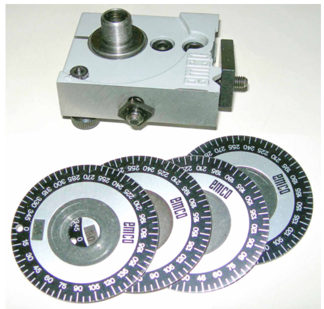
Unimat's dividing head also helped me make many of Optoform's pieces. This is compact, and versatile dividing head (only compatible with Emco chuck with 14 mm thread) that can be utilized to machine small parts.
