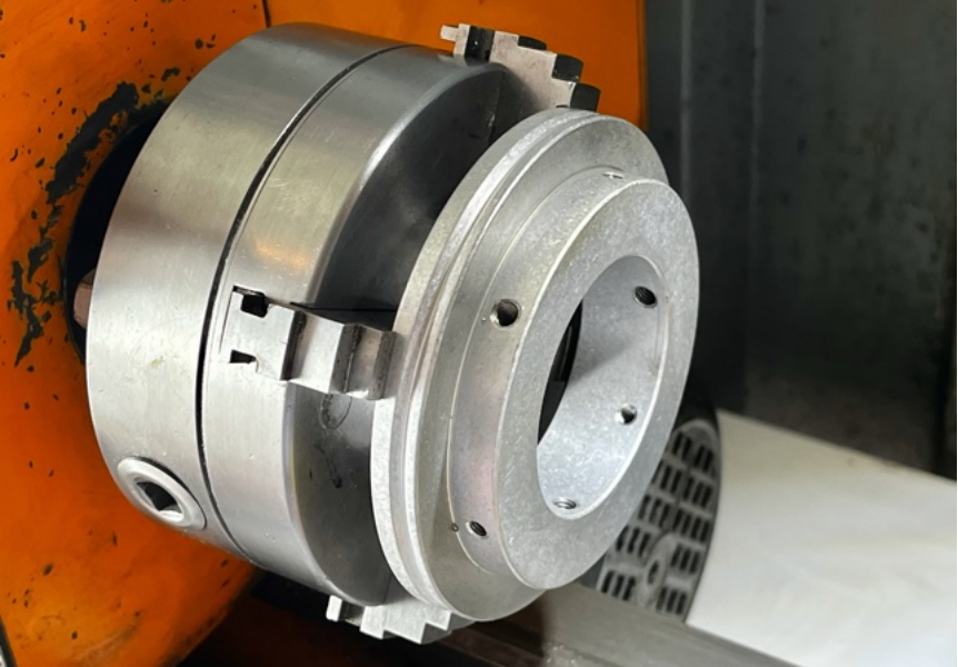
Soft jaws can be machined to hold specific diameters like above/below.
