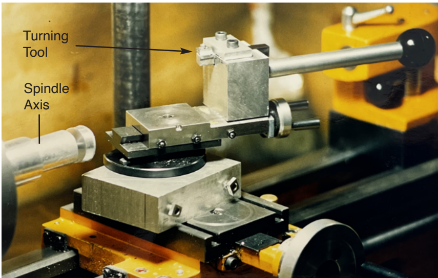
This fixture was built to machine Optoform's 50 mm spheres.
