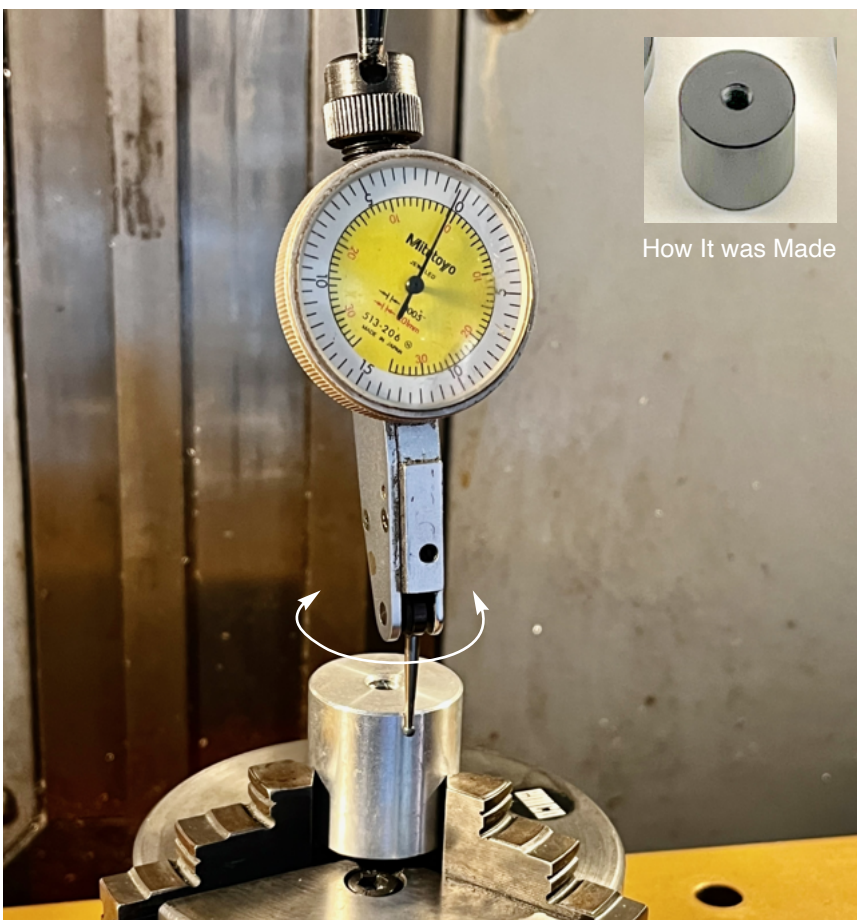
Centering the X-Y coordinates of a circular part using a dial indicator
