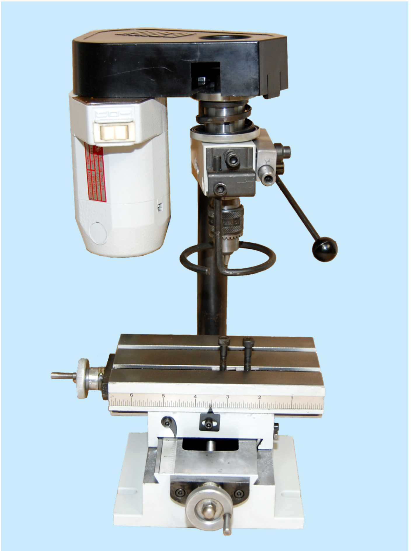
The precision hobbyist's machine. The legendary Unimat 3 on its optional X-Y milling table is a versatile table top machining center with numerous accessories for dividing, gear cutting, milling, drilling, and fly cutting operations. Over half a million Unimats 3's was sold world wide for their versatility, precision, and affordability.
