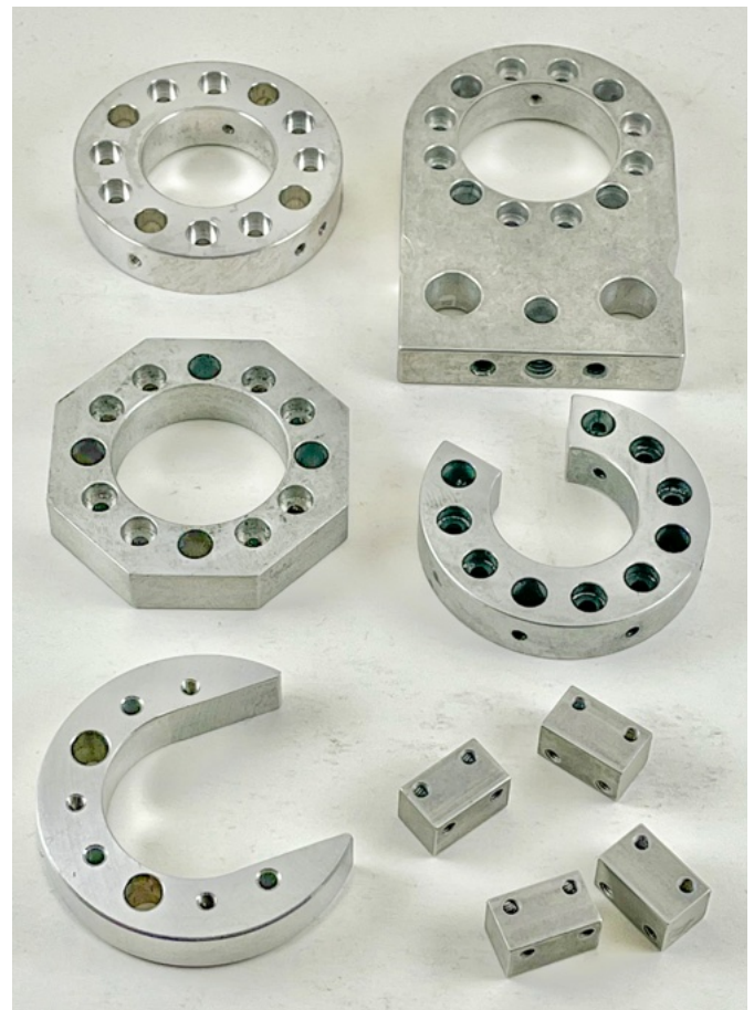
Unanodized Optoform pieces that I produced using Emco CNC Mill 50. Throughout this issue, I will show you how I made them for 10 years.
