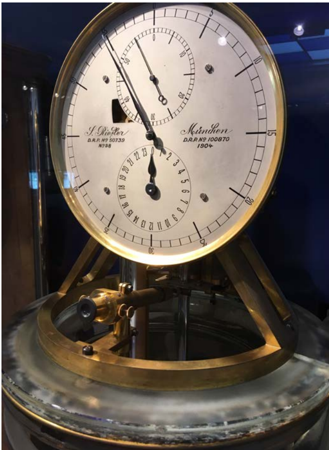
A precision clock made in Munich in 1904 (115 years old) with optical scope pointed at the stem of its pendulum. I saw this on many old clocks, including the Erwin Latter clock (bottom, right) that has a precise scale at its base.
