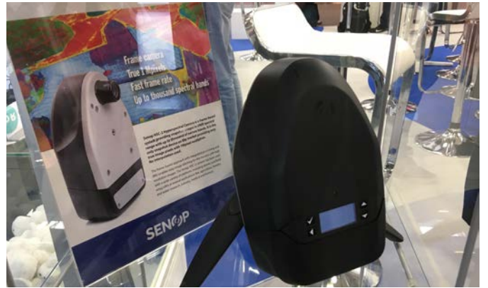
Multispectral camera by SenoP Oy Optronics Finland, provides 400-1000 nm spectral scan 1 Mega Pixel resolution.
