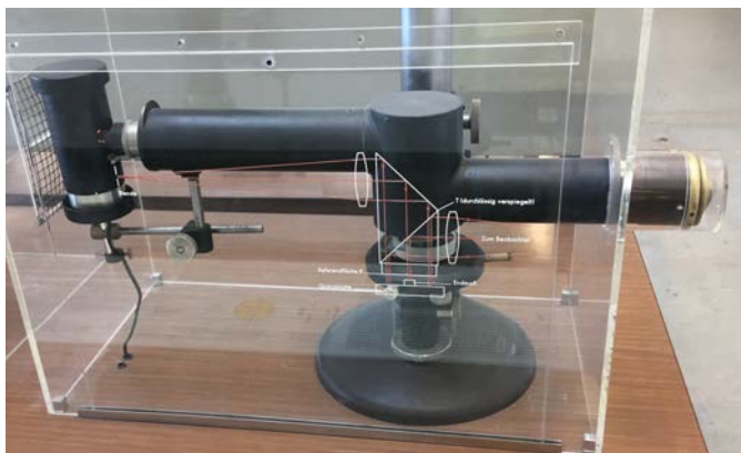
An interferometric comparator by Carl Zeiss Jena, 1921
