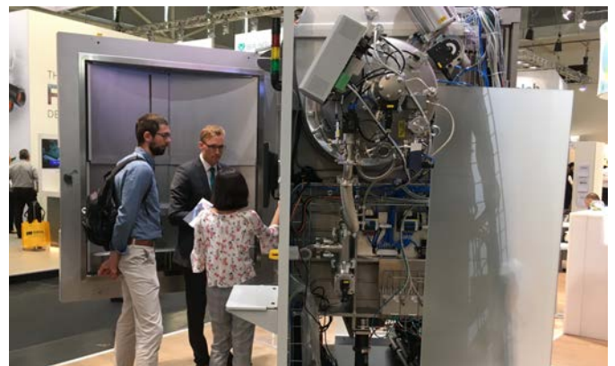
Huge optical coating chamber on display at Buhler Alzenau GmbH booth. Right, vacuum pumps/control electronics.
