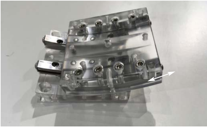
Roller bearing section of a goniometer stage by GMT Europe GmbH. They offer precision micrometer options (right)
